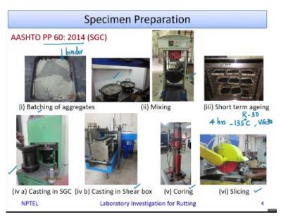
So for both these test, I will discuss how this specimen is prepared. The specimen is a cylindrical specimen of 100 mm diameter and 150 mm height. This is prepared as per the AASHTO protocol AASHTO PP 60. You decide the mix then you batch the aggregate first as per the required gradation.
