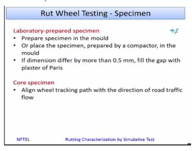
Now the specimen, you can have the specimen being prepared in the specified mould for the testing. You can use any compactor to compact the specimen to the required air void content. We normally do the testing at a 4% air void. So at this air void you can cast a specimen in the mould itself or you can cast the specimen using any other compactor. Say you can use a shear compactor to prepare the slab specimens.
