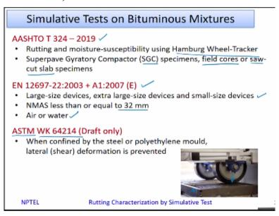
So there are various test protocols for a simulative test or a dry wheel tracker test. One is the AASHTO protocol which is AASHTO T 324, which uses a Hamburg wheel tracker for the testing wherein rutting as well as the moisture susceptibility of the material can be determined. So you can do the testing in the dry condition as well as in the wet condition.
