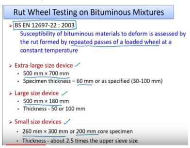
So let us discuss the European standard. So I will be discussing the rut wheel testing using the European standards. So I will read from the code. It says that the susceptibility of bituminous materials to deform is assessed by the rut formed by repeated passes of a loaded wheel at a constant temperature. So this is what is done in this test.
