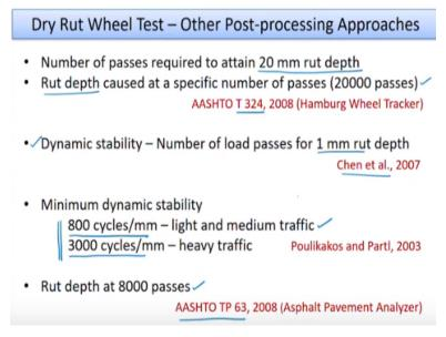
Now this is one way in which you can post process the data. There are other approaches by which you process the data and you set failure criteria for these materials. As per the AASHTO T 324 which uses the Hamburg wheel tracker the number of passes required to attain a 20 mm rut depth is taken as the criteria.
