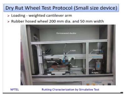
Now I will discuss about how the testing is done in a small size device in air. So this is a chamber or an environmental chamber where the test is being conducted. As you can see here, this is the bottom plate in which the specimen is kept. You can see the wheel here. And then the wheel load is applied using a cantilever arm.
