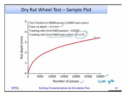
Now this is a sample plot of the rut depth versus number of passes. As you can see here, this is number of passes. So the test is continued for 30,000 passes or you can say that this is 15,000 cycles and you see the progression and the final rut depth that has reached that is this value is 3.4 mm and the tracking rate in millimeter plus 1000 load cycles you got it as 0.1175.
