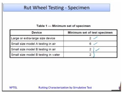
And you should have more number of specimens to check the repeatability. In the case of extra-large size device and the small size device you need at least two specimens to check the repeatability. Whereas in the case of, there is a small size device of type A in air it requires at least 6 specimens to be used.
