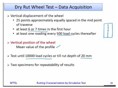
Now the test temperature based on your requirement, you have to choose the test temperature. So as we are discussing about rutting, rutting is something which happens at a higher temperature. So normally we do the testing at 50 or 60 degrees
