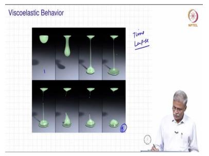
And in fact it can be very nicely explained by means of this kind of time lapse picture of a nice viscoelastic gel, actually you can see, if you go from 1 and all the way up to 8. You can see how the gel starts flowing, the thread gets cut. And then finally you can actually see how the shape exactly tries to recover, over a period of time. So this is more or less the response that we are going to see here.
