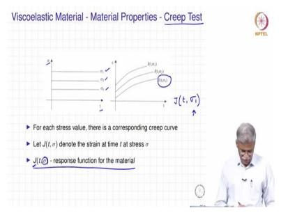
So we will do this Creep test. In fact, this particular test in which you apply a load  $\sigma$ , for a constant time t is  $\sigma_1$ ,  $\sigma_2$ ,  $\sigma_3$  is the creep test. And we are looking at the response of the strain. So I want you to take a close look at this particular function, J (t,  $\sigma_1$ ). So this function, basically tells
