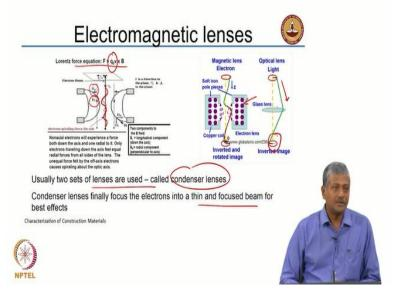
So once these electrons come down the optic axis, I said that you need to have these magnetic lenses to control the path of the electron so that they don't start straying out from central path, and move directly down the optic axis. So, from your high school physics, you may have come across this equation called Lorentz force equation and the idea is that as your magnetic
