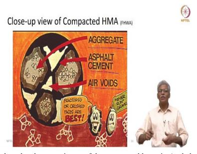
So, if you really look at the close-up picture of the compacted hot mix Asphalt, you are going to see the aggregate here, as you can see, and binder here and air voids here. So, when you use stones, of with fractured or crushed faces. They, you are going to get this completely better interlock.
