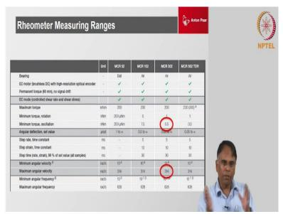
So when he the measure if we just looks at the specification of the instruments and he knows ok if I am measuring now the first data points of this measurements I am getting lot of noisy data. So first thing you should do this check the torque and see that torque is really in the range of the instrument many times the torque is so low and it is almost either lower than the capability of the instrument or very nearest to this lowest capability of the instrument ok.
