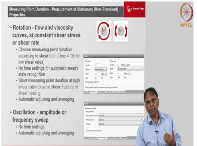
So, this is what you should really understand so when you are setting this parameters of shear rates okay take care of the timings that you are using if you are timing from low speed to high speed or low shear to high shear okay. So, you take a reciprocal of the time also let us am staring from 0.01 shear it to 100 shear it okay. Then I can start from the measuring time point see 120 seconds down to 5 seconds or 1 second we got 100 shear it overall in a fraction of second.
