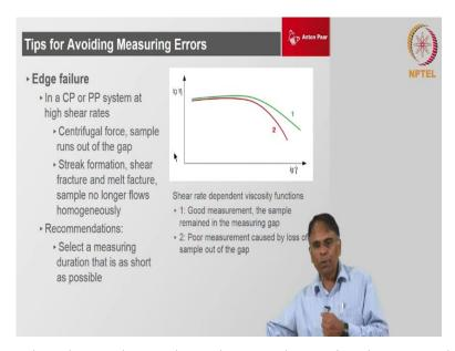
And we really need to know these where they are happening because otherwise, we start understanding that this is due to really the degeneration of the structure, but it can be due to the sample not getting hold inside the gap okay. So, the sample is not filling the gap at all and that is actually also crossing the fall of the modulus okay.
