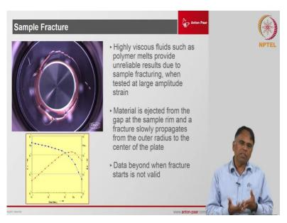
The other factor that is comes is the edge fracture, we can call it as a sample fracture. In simple terms if you have viscoelastic samples the when you are applying a shear on the samples the sample also develop what we call as a normal stress okay. And this normal stress is coming due to the you know Weissenberg effect. This normal stress will push the you know sample up but if you have a plate there is nowhere to go, so the only way the place to go is outside okay.
