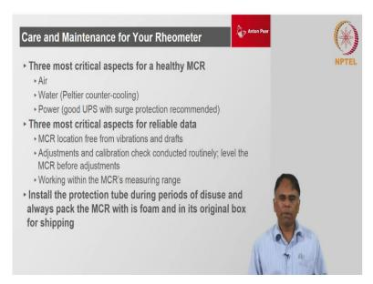
I would recommend at least once in 3 months or once in 6 months you should do the measurements. And then of course other things which are important to look at you are supplying air to the air bearing of this rheometer, so the dryers of this air bearing are important so keep on watching these dryers. They will be usually most of the dryers will have a color change as they get deteriorated.
