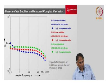
This is an example of an influence of a bubble if you have a bubble inside the sample you can see it will act like a particle inside a sample okay. It will give a same effect like a particle of the sample.
