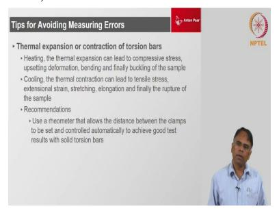
So, this is very good way to make sure that any temperature expansion or contraction is compensated by using this normal force control so of course this can be also used for bars.
