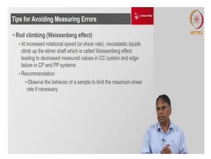
So other simple effects viscous-shear heating effects at very high shear rate, the Weissenberg effect at if you are using coaxial cylinder system, we can see sometimes the sample climbing up the rod this coaxial cylinder system okay. It can happen only in coaxial cylinder system not a parallel plate and cone plate. In the parallel plate and cone and plate it leads to edge fracture effect but in a coaxial cylinder system has the place to climb up it will climb up the rod.
