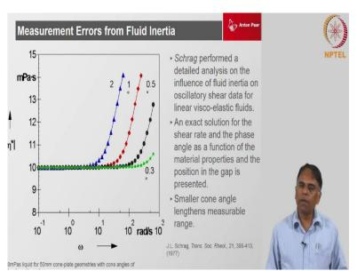
The secondary shear effect is nothing but you the material which was actually having a laminar flow it is goes into a turbulent flow okay. When it goes into a turbulent flow the layers which were actually flowing like nice laminar sheets, these laminar sheets actually are crossing each other now in a turbulent flow. And that is called crossing that extra shear and that is why you can see this viscosity increasing as a function of time.
