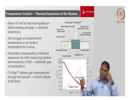
Also, the thermal expansion of this system have to be consider if you take cone and plate, then of course you cannot do a coaxial cylinder sorry you cannot do a temperature sweep with a cone and plate okay. There is a possibility of course which special geometry okay which will have senses in upper and lower geometries which can track the gap accurately then you can even do a temperature sweep on the cone and plate.
