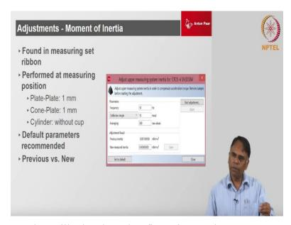
Both these things together will take altogether five minutes okay. So you required to put your tool without any sample to do a zero gap and do an inertia and motor adjustment either way you do a motor inertia or inertia and motor adjustment not a issue over here.
