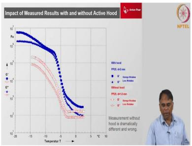
Example of the measurement between the same sample measure with the hood and without the hood you can see very big difference it is look like two different materials all together okay.
