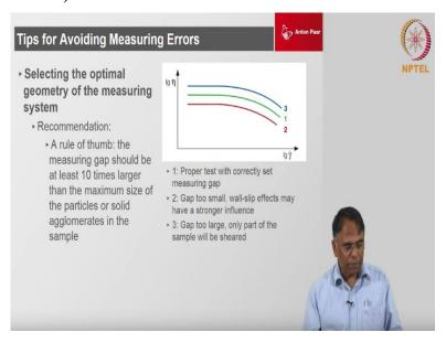
And then of course the particle size, as we were discussing if you have a particle size of 10 micron then the minimum gap you should is to be 10 times the largest particle size okay.
