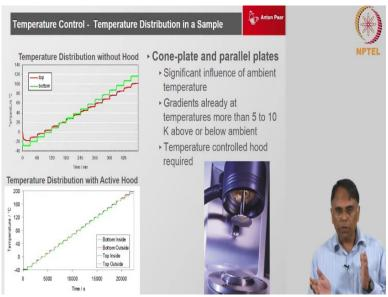
That case you can of course you can make these you know the adjusting time and averaging time to zero okay. You can still get very good measurements done using that parameters. Temperature control we have to also consider equilibrium times okay. Because the hardware's the geometry can heat up very fast, but the sample may not be heating up that fast. So always make sure that your sample is following the temperature steps that you are giving okay.
