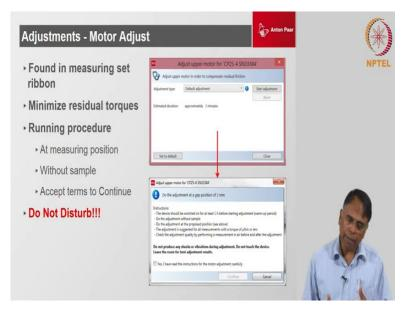
There are geometrics where if you are going to measure even the normal force then you can do a motor adjustment for a longer duration of time at very low shear condition so you can map not only the torque but also the normal force at all 360 degrees okay. If you do a long adjust it is actually both torque and the normal force and if you are doing short adjust generally only the torque will be mapped so this is what is done.
