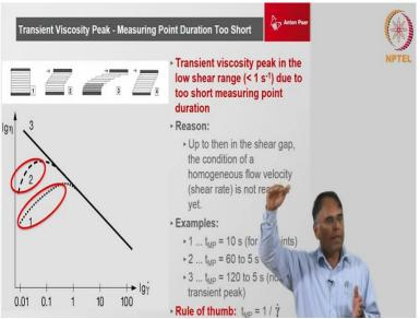
But if you want to do a non-transient experiment then of course you will require to get full you will have to give this sufficient time to make sure this complete aspect of adjusting recording and the application of the input parameter is done correctly over here. So, this is an example over here, see an example of a shear rate sweep ok if you have a shear rate sweep starting from 0.01 to 1 in the transient, you know with very short time you can see this banana curve ok which is happening okay.
