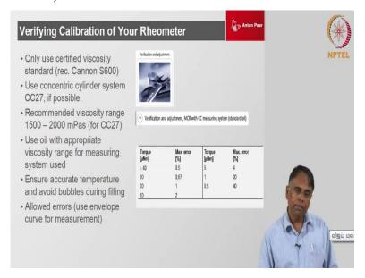
Temperature calibration is important, it has to be done once in a year at least and always cross check with either standard oil or standard reference material like a PDMS which has certain known values okay. Just to check that your measurements are really in the right place okay so this is something which also needs to be done on a regular base.
