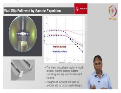
There are certain geometries that can be used for you know I would say not eliminating this but try to minimize effect of this or pushing against this effects too much higher strains okay. So, there is a geometry which we have you know cone partition plate which is generally used for this. Then the other you know artefact that get is the slippage between the samples. If you generally the geometries that we use very simple smooth surface is okay.
