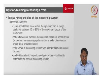
So, the pre shear helps, it is a very good pretreatment method over here okay and then of course the torque range and the size of measuring system. if you to find that the torque that you are getting of this especially the lower points is quite low okay at 25 mm geometry for example then you can immediately go for a 50 mm geometry that will automatically improve the torque at the small levels okay.
