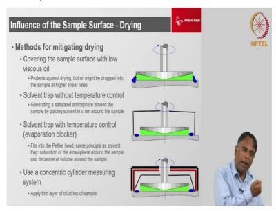
Then you have the drying effects, if you are measuring emuslions or dispersion or suspensions you can see the edge drying also gives us problems. So, if you have test which are long or you are doing at a little bit elevate temperature where there is a evaporation of the you know solvent phases inside there. So that can lead to that again you know wrong interpretation of the data you can see a moduli or you know a viscosity increases.
