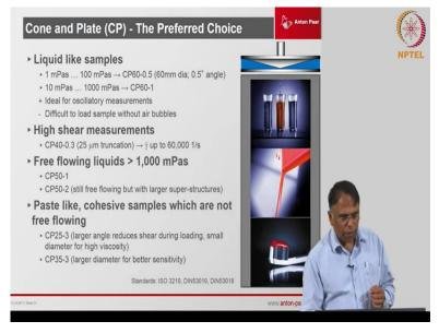
So, it is one of the most preferred choice of measurement and you can have so many varieties of geometries. If you want to measure very thin fluids you can have a small angle, if you have very strong structures you can measure a cone with large angles you can have different diameter different angles. So, variety of combination of cone and plates can be possible to suit any type of you know very wide variety of material I would say.
