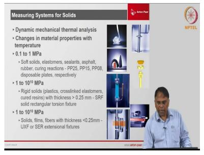
Then of course there are measuring systems for solid which I had told you that they are simple clamps ok. And these clamps can be of variety of type you can have solid rectangular fixtures for rectangular samples. You can have circular fixtures for cylindrical samples, and you can also have a holders for films and fibers also. So, this are something like this over here.
