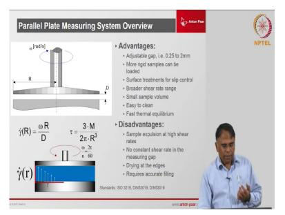
The other geometry besides the parallel plate ok it is one of the most adaptable geometry after cone and plate and the main advantage I would say for the parallel plate is easy sample loading and of course you can do temperature sweeps ok. Here we can do temperature sweeps because even if the gap is changing ok we can measure at any gap we can actually use that gap calculate.
