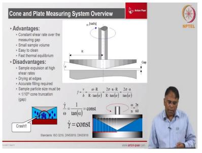
We have the cone and plate which is I would say one of the best geometries which can measure from low viscosities to medium high viscosities most versatile geometry I would say. It has lot of advantages because it has shear distribution across the surface which is constant from center to the edge ok. So, it is very good for it is good accurate measurement of viscosity using a cone and plate ok.
