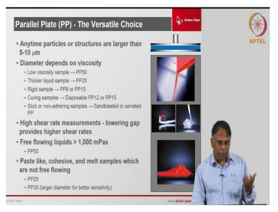
And also, since the parallel plate can be done at variety of gaps you can use 1 mm gap you can use 0.5 mm gap you can use 0.25 mm gap ok. So, the changeable gap basically also allows you to accommodate different type of samples. If you have samples of say with have particles as big as 10 microns then I can easily go to 10 times of that gap which is 100 micron and so on so. I can actually adjust the gap based on the maximum particle sizes which have present in the sample.
