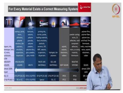
So, to choose you know proper measuring geometry for your samples you can just look at this surface area of geometry as a main parameter ok. If you have samples which are very weak very thin very structures like you know foams for example ok very so they are, the structural strength of this material is very weak.
