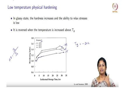
So what happens is that in the glassy state the hardness of bitumen increases substantially and the ability to relax stresses reduces. So this is very very important for pavements when the temperature falls below the glass transition temperature, this may not be very common in India. But imagine countries like Canada where the pavement temperatures can easily reach up to -30 or -40C.
