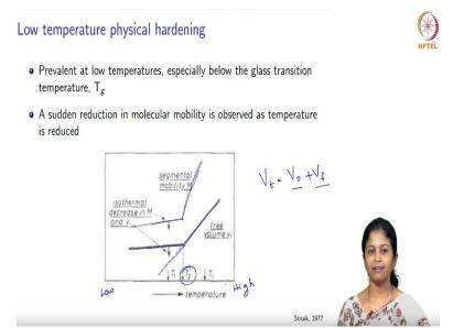
So what is this low-temperature physical hardening? So as the name suggests it occurs at low temperatures. So what happens is that when we reduce temperature from high temperatures with the reduction in temperature the molecules will try to reorganize themselves to form an equilibrium state or to attain an equilibrium state. So we can explain this in terms of a free
