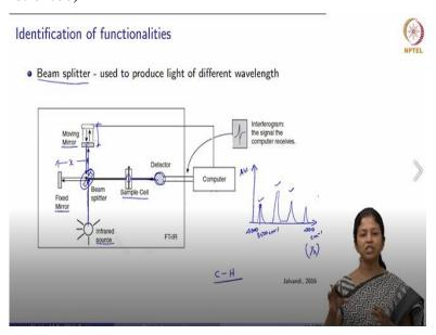
I will just explain in brief about this technique. This technique has a beam splitter, which is used to produce light of different wavelength. So, we see here, the first thing is we have an infra red source here. So, light is now input onto the beam splitter, right? This beam splitter splits this light into two different components. So, these two different components fall on a fixer mirror which is placed in here and then a moving mirror which is placed here.
