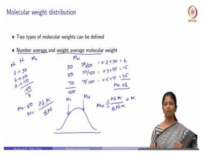
There are two types of molecular weight, so this is based on size. Now we have to calculate the molecular weight. There are two types of molecular weight that can be calculated for bitumen. A number average molecular weight, which is defined as M suffix n and weight average molecular weight, which is defined as M suffix w. When you look into the literature which talks about molecular weight for distribution you can see, they always refer to number average and weight average molecular weight.
