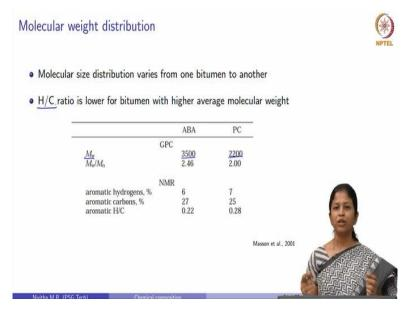
So this is one information from the study which we had seen earlier, we had seen the elemental composition for the same two type of bitumen. So we are going to see its molecular weight the number average molecular weight and the weight average molecular weight. So we see that for these two type of bitumen, the weight average molecular weight is higher for bitumen ABA, whereas it is lower for bitumen PC.
