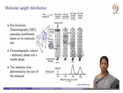
So to find out the molecular weight distribution of bitumen, we use a size exclusion chromatography. So this is a technique which is used to separate the constituents of bitumen based on their molecular size. So once we separate them based on the molecular size, we can calculate their molecular weight. So for this purpose, we use a chromatographic column.
