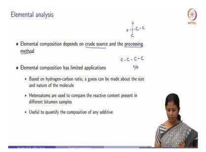
So what is this application of this elemental analysis? This has very limited applications as far as bitumen is concerned, it is very useful when we try to understand the hetero atom content which is present in bitumen and metal content which is present in bitumen. To see whether bitumen with higher metal content is showing higher viscosity or higher reactivity to certain conditions.
