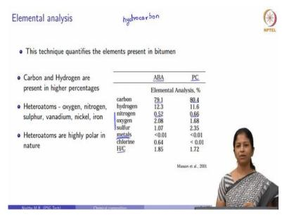
Elemental analysis says what this material is composed of at the elemental level. So we have different elements which are present in bitumen. I have shown you an example here of bitumen from two different sources. The first one is ABA and the second one is PC. So these are bitumen from two different crude sources. Let us see how the elemental analysis varies for each of these two bitumen.
