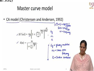
So now let us discuss in detail a CA model which is based on the research from as a part of SHRP path, Christensen and Anderson given this model CA model, you have 2 equations here describing a master curve for a dynamic modulus and master curve for a phase angle. Now, if you closely look into these 2 equations, so, you can see this either a dynamic modulus or a phase angle is a function of 3 constants, one is  $G_g$ , another one is or  $\omega_c$  and the 3rd one is R
