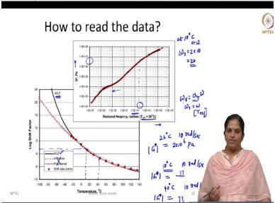
So, here is a master curve for a dynamic modulus. So, if Y scale is a dynamic modulus here and X scale is a reduced frequency. So, this master curve is constructed at a reference temperature of 26 degree Celsius. So, you have this master curve and that the master curve you have a corresponding shift factor. Now, let us not worry about the other shift factors, we will just take the WLF equation here, let us assume that the WLF equation holds for this master curve.
