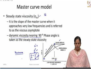
So, before we define a crossover frequency, let us just look into what a steady state viscosity. So, this steady state viscosity function though this is not directly included in that expression, we need to know what a steady state viscosity to understand what is crossover frequency ( $\omega_c$ ). So, now see
