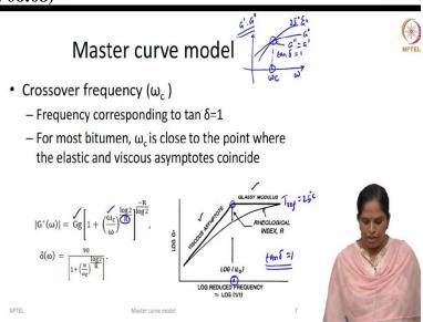
So, Glassy Modulus see generally if you see the master curve of dynamic modulus you have a schematic of a master curve here, in this schematic, you can see that the dynamic modulus master curve as plotted as a function of reduced frequency or it can be even an inverse reduced frequency, can also be imagined as a reduced inverse of time. So, you see a dynamic modulus curve here a master curve here at very high frequency.
