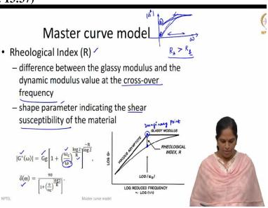
It is called as a rheological index. So, this rheological index is nothing but the difference in the modulus value obtained at the crossover point. So, we have a crossover point here so, modulus value obtained from this peak point to the modulus value which we get it here. So, this point is an imaginary point. So, this is the one which we get it from the master curve. So, difference between the glassy modulus which is a straight line here.
