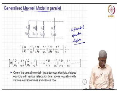
So, you can also have the Generalised Maxwell model in parallel and you need to have what is really called as the, to solve such kind of problems, you need to have what is really called the differential operator algebra, I am mentioning all this things in passing because we are still working with linear viscoelasticity and we are not even talking about nonlinear viscoelasticity.
