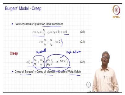
So if we need since we have second order equations, we need two initial conditions when we write the initial conditions like this at t is equal to zero and similarly, we also have to impose this initial condition as for as the Kelvin model is concerned. And when we try and solve it here. This is the expression that we are going to get. I have not made a mention of how this has to be solved.
