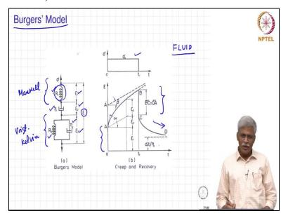
So what we are now going to do is we are going to combine them two. So, we are going to see that there is a Maxwell model and there is a Kelvin model and we are going to combine them in series. This is one of the well-known model that has been used for characterizing the response of bituminous binders, bituminous mixtures, polymer gels, blood and many other fluids that are available.
