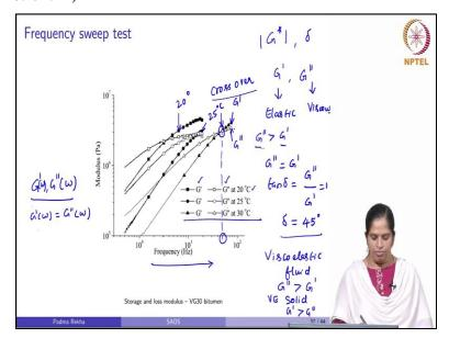
So, as we know that when you do an oscillatory shear testing we either measure a dynamic modulus and phase angle. We need a minimum 2 parameters to define one it can be a dynamic modulus and a phase angle or storage modulus and the loss modulus. The storage modulus represents the elastic response and the loss model represents the viscous response. So, we need 2 material functions to define a viscoelastic characteristics property of a material.
