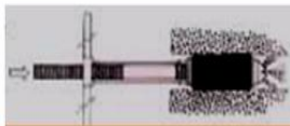
STEP 2: The packer is expanded in the hole using the tightening lever. Injection can then start.
