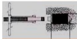
STEP 3: When the injection is finished, the valve closes itself. The injection lance is disconnected by un-screwing the tightening lever, while the rubber sleeve on the packer remains expanded.
