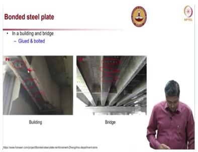
Now in a building, example for a building you can see here there are bolts provided, whatever I just showed in the previous slide. And here also you can see a lot of rivets and which is provided to hold the plate and then facilitate injecting grout into this place. I mean first you will anyway provide some glue there or adhesive but if required we can also go the other way by injecting into the space between the plate and the concrete surface.
