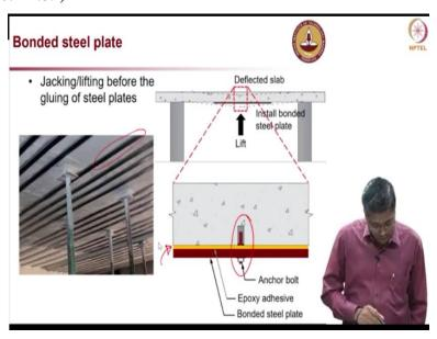
So steel plate, you can see an example here. This picture I showed it is not a steel plate, it is a CFRP laminate here, but I thought this is a good photograph to show you how this process
