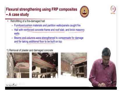
Now I am going to show a case study where this FRP laminates were used. This was actually a building, which had fire incident and basically like a lot of furniture, cushion materials, partition walls, panels, etc. were actually functioning like the fuel for the fire and it lasted for a couple of hours. And then the hall with RC concrete frame, roof slab and brick masonry walls; they were all attacked by the fire.
