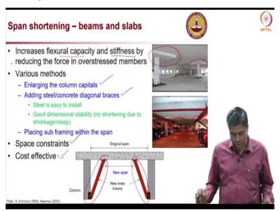
Now span shortening is another widely used practice to enhance the flexural capacity. Not only capacity, it also helps in enhancing the stiffness of the member by reducing the amount of stress
