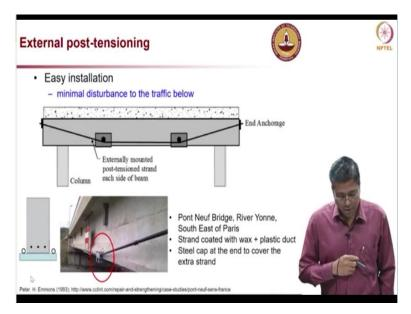
Now next way by which flexure strengthening is done is external post-tensioning. I am going to show some examples on this too. You can see here an anchorage; a tendon is placed like this, these are the deviator blocks and this black line indicates the additional tendon. Photograph at the bottom very clearly shows the tendon here and it goes like this and goes up on the other end of the bridge and this is the deviator point there.
