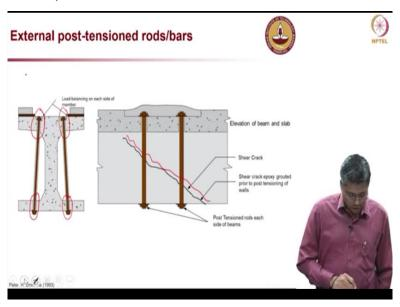
This is the external post-tensioning, because drilling that hole if it is a deep beam, it is a lot of work and sometimes it is not very easy and practical. So in such cases, we can go for external post-tensioning where drilling is required only for this much length very short amount of work and then you connect either a rod or a strand or a cable system, so that the shear resistance can be enhanced.
