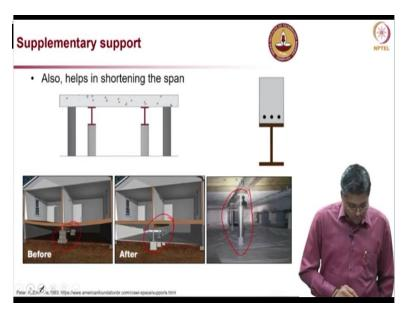
Now next is supplementary support system, where we are talking about structures which might have significant deflection and which need to be strengthened. One example is, look at here in the bottom left two images before and after, you can see there significant deflection and then that deflection can be nullified or the whole system can be jacked up by using some supplementary support systems. You can see here this is an example photograph; it is a jack where the height is actually adjusted.
