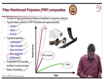
Now let us talk about fiber reinforced polymer composite. It consists of high-performance fibers, very strong and very stiff fibers embedded in polymer matrices. So you can see the stress-strain graph of fiber which indicates high strength and stiffness which is embedded in a resin, which
