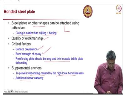
Now bonded steel plate, let us look at steel plates first and then we will talk about examples of FRP laminates. So steel plates or other shapes can be attached using adhesives. Other shape are, I
