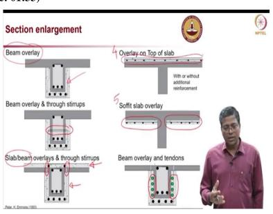
First let us look at section enlargement. I am showing here six different ways by which we can enlarge the section and enhance the flexural resistance. In all these drawings the dark gray region
