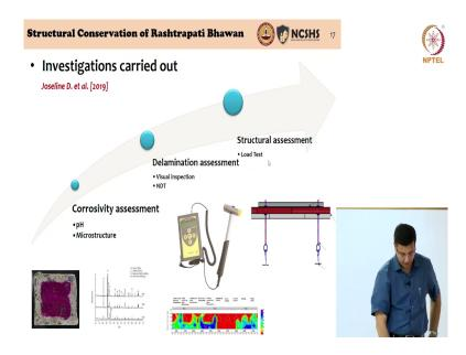
So, again some investigations had to be carried out. We had to understand how much of corrosion is happening and because of corrosion in the steel there was damage to the material and that had to be assessed. They then had to understand, it is 1.2 kilometers of sun shades; we could do a test in one location, but it may not be representative of another location.
