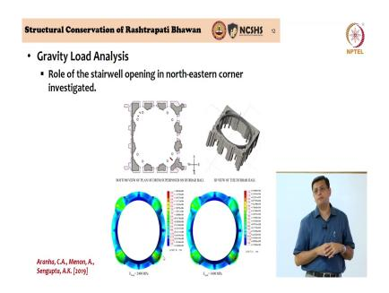
So, this is a section of the plan, cut section of the finite element model; we basically looked at what is the role that this stable opening was playing and it actually showed us that the presence of it was what was creating these tension cracks. Now, having understood what the problem is, we can now comfortably work on a solution; because we did not want to work on a solution without knowing what was happening, then you may be completely going wrong, right. So, this was the first aspect.
