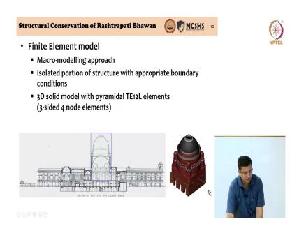
So, we actually had to now understand in a more detailed manner why this was cracking. So, it is a complex structure and therefore, while we do some basic hand calculations; we also depend on some complex computer based simulation, so that the behavior of the structure can be understood in a more rigorous manner.
