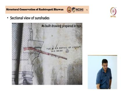
And we had original drawings. So, we went back to the original drawings, but in the original drawings, we saw somebody had made some correction, ok. So, as per Lutyen's design, Edwin Lutyen's the original design these were meant to be Chhajja's like in the Rajasthani architecture. If you have seen, there are large cornices and sun shades made out of sandstone; that are present in big buildings in Rajasthan in Western India. These people had drawn inspiration from ancient Indian architecture.
