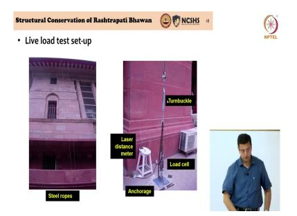
So, this is just a picture of the load test, we are pulling these sun shades down to simulate the weight of people standing on it and working to put the lights and take them off later.
