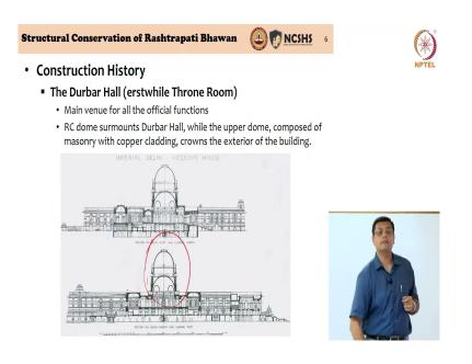
So, that is the original drawing, it is it was a good thing early 1900s; we had Edwin Lutyen's drawings and these drawings were on cloth. So, they would be as large as a room, you spread it out on the floor and you have all the details measured drawings. And so, we could look at the original designs and then look at what was constructed in the building and see if they were deviations and start understanding why the structure developed some damage.
