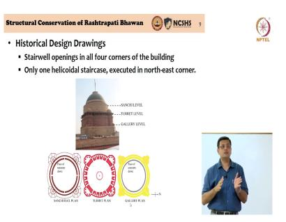
There were four spiral staircases intended in the structure in all four corners of the dome. But when the construction was completed there was only one spiral or helicoidal staircase that was constructed; whereas the other three locations did not have these spiral staircases.
