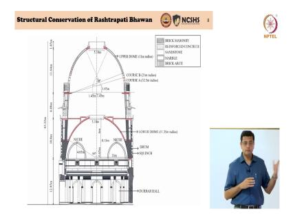
Now, on the north eastern and the north western corners where I have highlighted them in red, those two niches in the dome had cracks. One of the niches has a significant crack, you can see the red line here super post on this picture and on the other side there are two smaller cracks.
