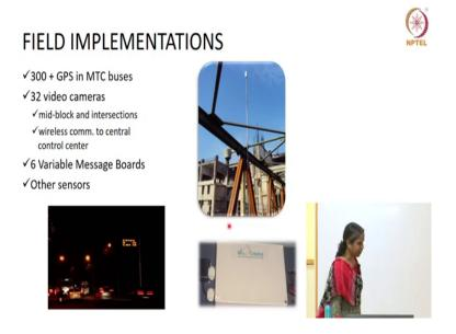
So, the complete cycle we have implemented in a this small corridor. What are all the sensors, we have around 300 MTC buses with GPS sitting and sending the data to our lab every 5 seconds or 10 seconds. We have around 32 video cameras relaying their feed to our lab. So, then we have message boards which we have installed in the field which gives information back to the users and there are other several sensors which I have enlisted.
