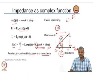
So impedance can also be represented on a complex plane by the use of these Euler relationships.  $\exp(j\phi) = \cos\phi + j\sin\phi$
