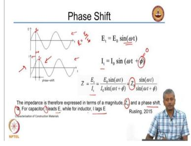
So first of all again one of the common aspects of understanding impedance is that the impedance is not always in phase with the current. You know very well about phase shift with respect to waves, you can have waves that are in phase or out of phase. So for the waves to be in phase you should have an exact difference of  $n\lambda$  between the wavelengths of the waves; any waves that are  $n\lambda$  apart will be in phase; if you have  $(n\lambda/2)$  they will be completely out of phase.
