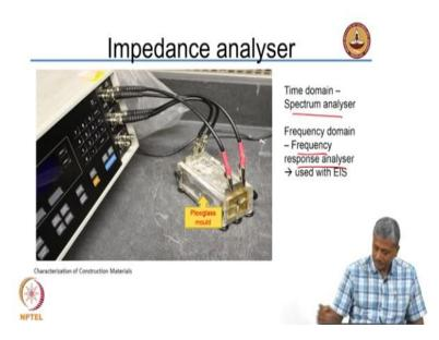
This is your impedance analyzer which is typically used - this is the one from our lab. So in the impedance analyzers which are also known as spectrum analyzers when they do just a time domain analysis, whereas when you do a frequency domain analysis which you typically get with most modern EIS systems, you call it a frequency response analyzer.
