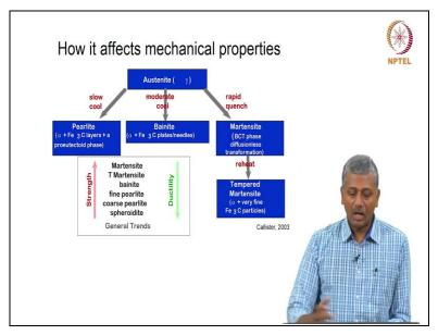
So how the composition affects mechanical properties, austenite on slow cooling can form pearlite, in moderate cooling it forms bainite and rapid quenching it forms martensite. So, if you go from pearlite towards martensite, your ductility reduces but strength increases. But what you can do is take the martensite and reheat it and then cool it slowly, you do not reheat to above austenitic temperature because then that will convert to austenite again.
