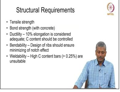
Of course you also have structural requirements for steel, you need obviously the tensile strength, which is the primary characteristic as a reinforcing material. You need to have a good bond with concrete because of which the ribs are introduced into the steel and ductility is important because we need sufficient level of ductility to get the performance of the structure that we desire. 10% elongation is usually considered adequate but typical steels will give you close 20% elongation.
