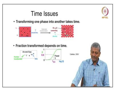
Now it does not end with that. We know that steel is formed in molten state and then cooled to the solid. The time over which this transformation takes place determines actually what the microstructure which is forming, but earlier we saw that there is a eutectoid transformations that assumes one important thing that - there is equilibrium during this transition. That means you have infinite time over which this transformation is happening from above 727 to below 727.
