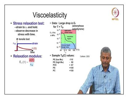
And again why I wanted to say that you need to consider these characteristics is the extent of temperature is different for these different polymers. For example if we consider PVC - polyvinyl chloride, what is a common application of PVC; pipes carrying water. So it has a glass transition temperature of 87 °C. What is the relevance of that? What is the significance of that? So when we have extremely hot water, we do not want to use polyvinyl chloride.
