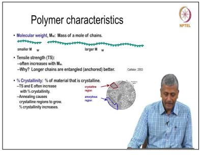
So, again, there are several indicators of the performance of the polymer, you have molecular weight, which indicates how many links are connected together. Tensile strength increases with the molecular weight and again percentage of crystallinity is defining the material that is crystalline. So if you look at the polymer under the microscope and recognise how many of the regions are actually looking ordered, that is basically your degree of crystallinity in the polymer.
