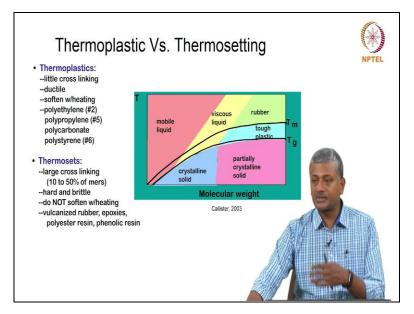
So because of this, we have different types of performances exhibited. You must have learnt about thermoplastics and thermosetting. Thermo setting is essentially your cross-linked and reticulated Polymers. Thermoplastic means linear and branched, which are easily able to move when temperature is increased.
