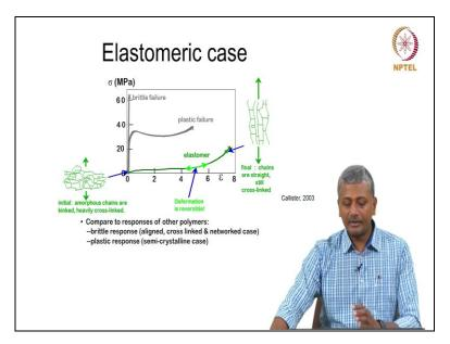
And there can also be another case called elastomeric case that is just like what we see in rubber. In rubber what happens is at very small level of stress, there is a very large recoverable strain and mostly the stress-strain relationship is non-linear. You see the stress strain relationship of rubber, at very low levels of stress and of extremely high strains which can be recovered but then it is non-linear; the stress strain behaviour is essentially non-linear.
