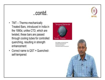
TMT which is otherwise written as thermo mechanically treated bars were introduced in India in 1990's. So, here what happens is these bars, actually any bar goes through a thermo mechanical process. So, actually this is not the correct name. The correct name is QST or quenched self tempered bar. Thermo mechanical process means any bar goes through a temperature treatment and some mechanical treatment - that happens for anything.
