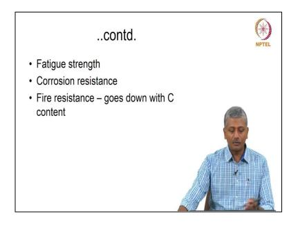
Of course other important characteristics include fatigue strength, corrosion resistance and finally fire resistance. Again fire resistance goes down with carbon content, the higher the carbon the lower the fire resistance.
