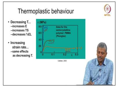
And what happens to thermoplastic materials when you have change in temperature and you test the mechanical response at 4°C degrees you get something like this and at 40°C, it is here at 60°C is here. You can see that there is a major drop in the ultimate stress levels when you increase the temperature. So, thermoplastic materials are extremely dependent on the temperature.
