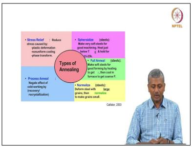
And in case of martensite you have this tempering process, which we just saw. Again within annealing itself we got different types of processes which need to be studied in detail to really figure out what ultimately we get in the steel.
