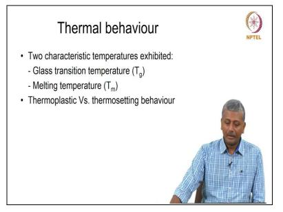
The other important characteristic is obviously the temperature behaviour. Polymers exhibit 2 typical temperatures one is called a glass transition temperature  $(T_g)$  and other is the melting temperature  $(T_m)$ . And because of this we also classify polymers into different types; we call them thermosetting or thermoplastic polymers. Now a purely amorphous polymer will only exhibit glass transition temperature. A purely crystalline polymer will only exhibit melting
