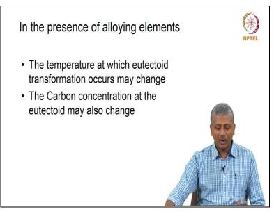
So when alloying elements are used in steel, (Nickel, chromium, sometimes copper are used to increase the corrosion resistance of the Steel), what happens is these may shift the temperature at which eutectoid transformation occurs, and the carbon concentration also may shift a little bit, when some alloying elements are built into this system.
