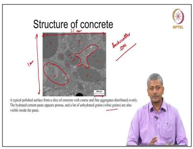
This is a structure of concrete imaged with the help of Backscatter SEM. We'll talk in detail about this technique later. But this Backscatter SEM technique was used to actually determine this internal structure of the concrete. So you can here see the aggregates which are present. Some are large, some are small, and this size is 200 microns. So the overall field width is about, this is probably about, 1.5 millimetre (X-direction). It is quite small still.
