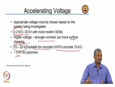
The electron beam speed is controlled by the potential difference that is applied between the electron gun and the anode. So that controls the electron speed. The movement of the stage up or down only controls the working distance, that is the distance between the objective lens and the sample.
