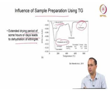
Also we can use this thermogravimetry to find out the influence of sample preparation. It depends on the material, right? So in this case, if you want to evaluate the effect of drying, for an example, what happens when you dry the sample? So (Refer Figure in slide), this is 1 day drying at 105 °C this is 30 minutes at 105 °C, this is no drying. So these effects can be evaluated.
