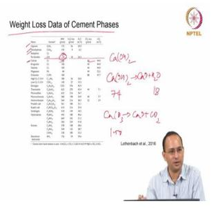
So here is a table you can use for the weight loss. This is the weight loss data of cement phases, starting with gypsum, hemihydrate, anhydrite, let us look at the portlandite. So, in portlandite, molecular weight is 74, add respective molecular weights of calcium, oxygen, hydrogen. And then how much water will you lose? 18 grams. So what is basically happening is:
