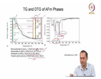
Similarly if you look at the AFm phases, we are talking about monocarbonate, monosulphate phases. And additionally you have this Friedel's salt is also there, which is a chloride form. So you are losing water at different temperatures, so let us look at the left plot (on slide).
