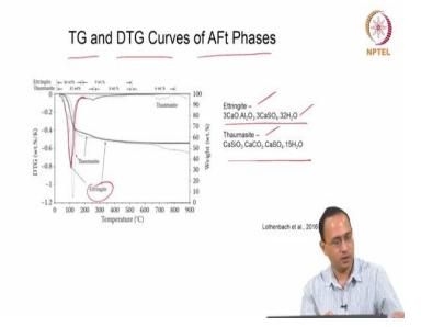
Now, if you look at the TG and DTG comes for AFt phases, AFt phase means in this case, we are looking at ettringite, thaumasite, right? The formula is:
