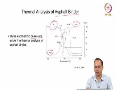
Thermal analysis can be also used for asphalt binder; this is one example where you use the TGA. So you see here lot of things, first TG curve is there, so the blue one (in figure) is TG curve, you see the continuous mass loss by around 600-700°C it is almost zero, everything is lost nothing is left, you see almost 100% weight loss. This is the TG. Now this is the DTG - change in slope (blue line). Then this is the DTA (green curve).
