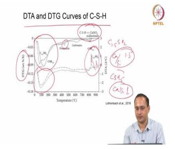
Okay, so here now it is a DTA and DTG curves of C-S-H, if you look at pure C-S-H, calcium silicate hydrate phase. There is no TG, but it is DTG, which is the first order derivative of TG curve, so you see this primary region again because of the loss of water from C-S-H here they have used two different types of C-S-H; one is  $C_{1.5}SH_2$  which corresponds to calcium to silica (Ca/Si) ratio of 1.5 and the other is  $CSH_{1.5}$  which corresponds to Ca/Si ratio of 1.
