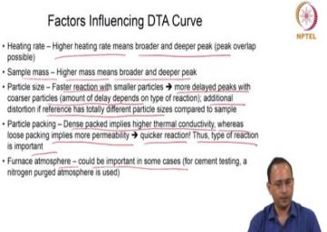
Heating rate means higher heating rate means broader and deeper peaks, peak overlap is possible for this case. You may get endothermic peak and exothermic peak depending on the temperature change. So when you have increase in the heating rate it means your peak will be broader and deeper. One of the factors influencing is sample mass; higher mass means broader and deeper peak.
