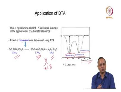
So, I will give you an example, so one of the most celebrated example of the application of DTA to material science is the use of high alumina cement which in some circumstances led to the weakening and in extreme cases to the collapse of concrete structures. So high alumina cement was used 30 to 40 years ago so at the time, these issues were observed.
