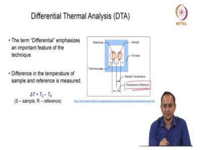
For differential thermal analysis, the term differential emphasizes an important feature of the technique. In this we measure the difference in the temperature of sample and reference. You have a reference along with your sample and as you are heating your sample and reference together; you measure the difference temperature difference that is the key concept.
