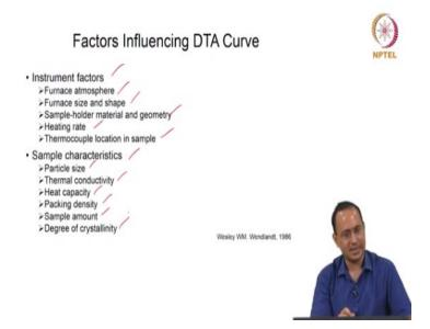
Now let us look at the factors which influence DTA. So, we know how to measure the temperature using thermocouples. If you carry out an experiment it is important to look at the instrument factors like furnace atmosphere, furnace size and shape, sample-holder material and geometry, heating rate and thermocouple location in sample.
