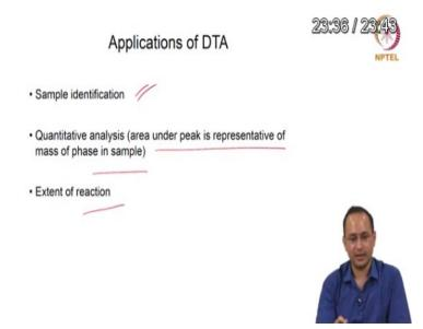
Applications of DTA are sample identification, because you can identify samples as they will have a particular signature. Dehydration is an example as it is dependent on the phase as it has particular signature. Quantitative analysis, where area under the peak is the representative of mass of phase in sample. Also extent of reaction or the degree of reaction can be calculated, this is among the application of DTA.
