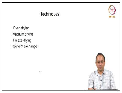
There are different techniques for hydration stoppage including oven drying, vacuum drying, freeze drying, and solvent exchange. In oven drying, you are simply putting sample at some high temperature remove the capillary water so as to stop hydration.
