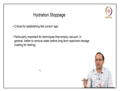
One of the most critical steps in sample preparation is hydration stoppage. We need to know the reason for stopping hydration. We mix cement and water and let it hydrate and during the hydration there is formation of calcium silicate hydrate and other cement hydrates, which continues and contributes in gaining strength. It is critical for stabilizing the correct age.
