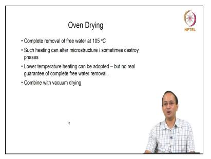
Oven drying is complete removal of free water at 105 degree Celsius. If you treat your sample i.e. cement paste or concrete at 105 degree Celsius then you will remove the capillary water. But the key issue with this method is heating at this high temperature can alter the microstructure and sometimes destroy phases.
