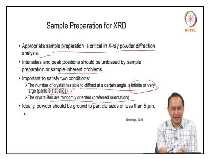
So, appropriate sample preparation is critical for x-ray powder diffraction analysis. Intensities and peak position should be unbiased by sample preparation or sample-inherent problems. You do not want to adopt a sample preparation which affects your sample.
