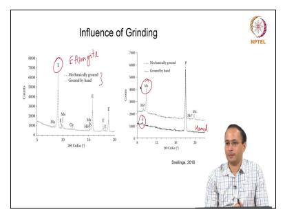
For example we take cement paste sample. X-ray diffraction plot for the cement paste sample is shown. So here the comparison is drawn between mechanical grounding and grinding by hand. E in the plot is basically Ettringite which is one of the phase in hydrated cement paste.
