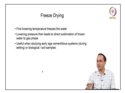
In freeze drying, you first lower the temperature so that the water freezes. Now, lowering pressures can be used to direct sublimation of freeze water to gas phase. That is how we are removing the water. So it is useful for studying early age cementitious system during setting. Suppose, you are interested in hydrated cement behavior in the early hours of setting you use this method. Freeze drying is also used for biological /soil samples
