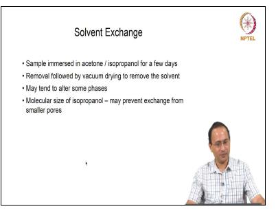
Most commonly used technique is solvent exchange. In this technique, sample is immersed in acetone or isopropanol for a few days. The main idea is alcohol will mix with water as it is immiscible liquid and then we remove it by vacuum drying. So vacuum drying is used to remove the solvent. It may tend to alter some phases.
