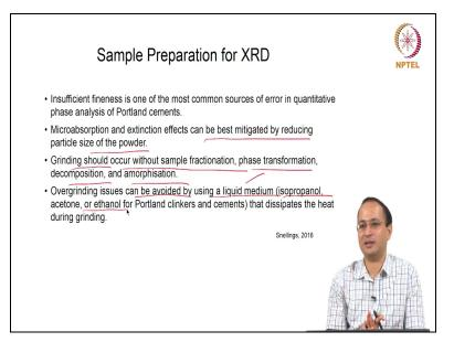
Insufficient fineness is one of the most common sources of error in quantitative phase analysis of Portland cements. Microabsorption and extinction effects can be best mitigated by reducing particle size of the powder. So you have to make sure of using fine powder.
