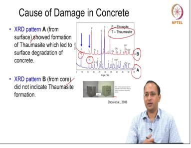
X-ray diffraction is commonly used technique in construction materials and it can be used to determine or identify the cause of damage in concrete. In this example, what we see in this plot, two x-ray diffraction patterns of samples - one taken from core and one from surface. Obviously one from core did not have any damage; but one with the surface had the damage.
