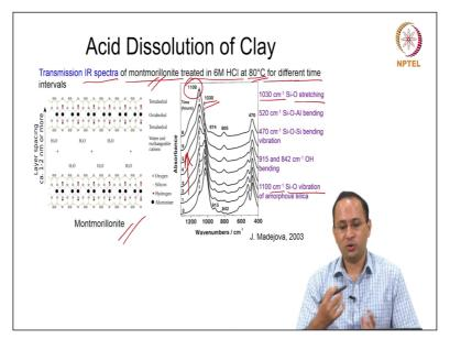
One of the techniques which will be covered in the class will be Infrared Spectroscopy. So, in this case, the transmission IR spectra can be analyzed and used to monitor the changes in montmorillonite clay (a type of clay), when it is exposed to 6M hydrochloric acid at 80°C, for different time intervals. So, you have the structure of montmorinollite in the figure.
