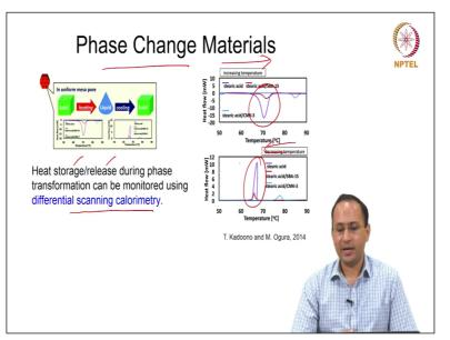
We earlier talked about Heat Signal. We can also quantify how much heat is absorbed and how much heat is released. So, basically heat storage and release during phase transformation can also be captured using the Differential Scanning Calorimetry. So, you might have heard of phase change materials.
