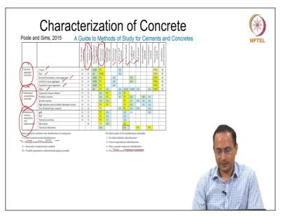
So, as far as characterization of concrete is concerned, there is a guide to methods of study for cements and concrete. What kind of methods can be used and what is the limitation. So, in this table, we have concrete aggregate materials in the first column, unhydrated cement and mixtures and replacement. If you want to study these materials, aggregates will be coarse, fine, recycled, artificial fillers.
