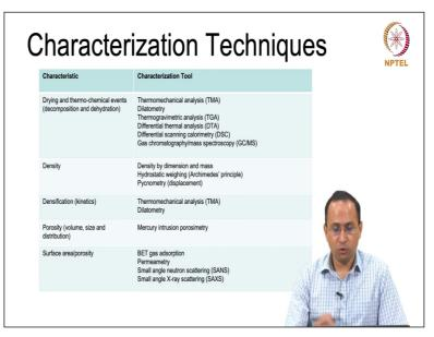
If you are looking at drying and thermo-chemical events like decomposition and dehydration, we can use Thermomechanical Analysis (TMA), Dilatometry, Thermogravimetric analysis (TGA), Differential Thermal Analysis, Differential scanning, Calorimetry, Gas Chromatography, Mass spectroscopy. So, these are the techniques which we can use for drying and thermo-chemical events. Similarly the technique, the characteristics and corresponding characterization tools which are available have been listed.
