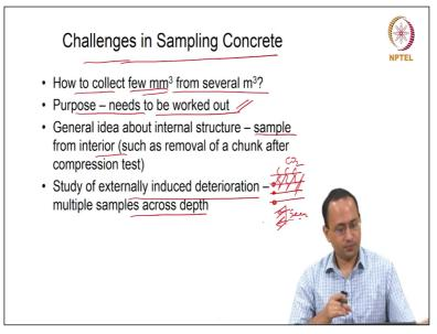
There are challenges in sampling concrete. It is not that easy because we want to get information of concrete, which is in structure. So, how to collect small amount of concrete from large? If we are talking about a structure, means we are talking about either a building, road,
