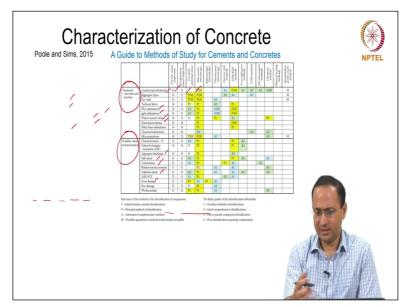
Here is another table. Now, we are looking at Hardened concrete and mortar so what type of cement, cement types, aggregate types, air void, admixtures, GGBS, water/cement ratio, pozzolans. And then, we are also sometimes interested in various type of degradation mechanisms - ASR, sulphate attack. So, this, gives us some information as to what kind of techniques, we can use for better characterization of concrete. So it can serve as a guide to various methods to study cements and concrete.
