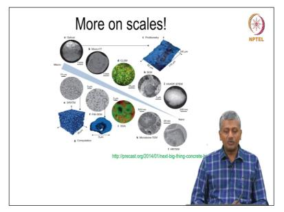
Again we can take this discussion of scales for any number of materials. But here again there is an example from concrete. So, what type of processes are applied at different types of scales so you have here you have optical microscopy Micro computed tomography using x-rays and then you have SEM and scanning tunnelling microscopy and high resolution transmission electron microscopy.
