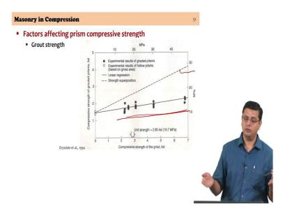
And finally, examining the grout strength; so, if you looking at hollow grouted masonry and if you were to again grout the void we are not looking at reinforced in this case it is just the hollow block with grout, what you see is that the effect of the grout is it is there it is weak right.
