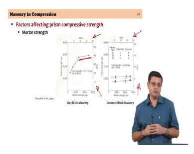
If you are looking at the role that the mortar strength will play on the compressive strength of the masonry assembly what comes out as an important message is beyond a certain mortar compressive strength you cannot increase the prism compressive strength. There is a saturation; it does not mean that you keep increasing the strength of the mortar you going to get stronger and stronger unit stronger and stronger masonry, there is a saturation that happens.
