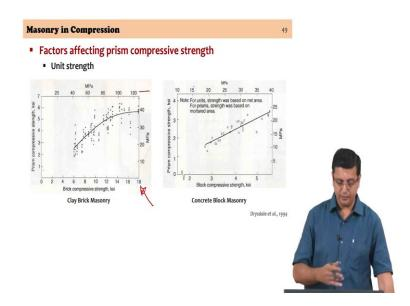
The unit strength how about the unit strength you are again looking at clay brick unit compressive strength on the x axis (MPa) on the top and the prism compressive strength on the y axis you can see that it definitely has a very significant role in the compressive strength of masonry, again significant or steep increase and then saturation beyond certain level.
