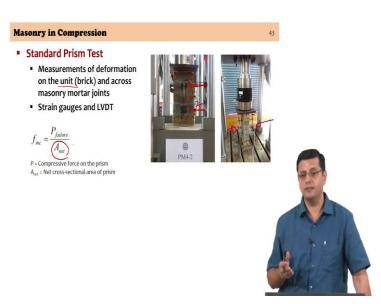
So, what is important is that you have measurements of what is the strain or deformation in the brick. So, you will have strain gauges fixed on to the brick unit itself, but if you want the deformation in the masonry you need to have measurement across at least one mortar joint and that is what you see here.
