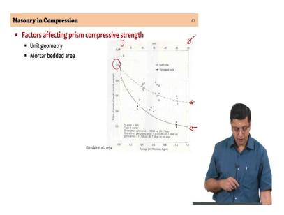
Let us examine a few factors that affect the compressive strength. You are looking at the unit geometry and the mortar bedded area. So, primarily what is the kind of role the unit geometry has or the mortar bedded area has if you are looking at solid blocks versus perforated blocks right. The gross area versus the net area effect as far as the strength is concerned.
