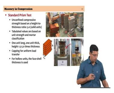
In terms of the test method itself, a standard prism test is what is conducted and now we are really looking at an unconfined compressive strength test. The unit is subjected to; the stack of bricks with the mortar subjected to uniaxial concentric loading.
