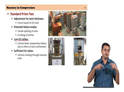
If you are unable to carry out a test with prescribed values of h/t adjustments for the joint thickness or the number of layers of bricks or units in the stack can be carried out by factors typically given to you in codes. So, we look at; we look at the differences that are
