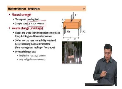
Again, compressive strength is one of the properties that you would check, but you also need to know the flexural tensile strength, the tensile strength of the mortar sample. Three-point bending test as we had looked at; the three-point bending test for the brick unit can be adopted here.
