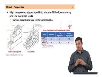
So, that brings us to two sets of constituents that we talked about and as I had mentioned earlier, grout is another important constituent of masonry construction today. The hollow blocks partly are grouted or sometimes fully grouted and when you have reinforcement, you have to grout the cavity in which you the reinforcement. So, grout itself is a different material.
