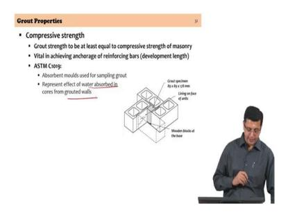
So, again since it is a property that can alter the strength of masonry, a check on the grout property, grout's compressive strength is one of the minimum tests that is carried out to characterize the grout itself. So, the grout compressive strength, we expect it to be at least equal to the compressive strength of the masonry, of the assembly right, it will work out to be close to the compressive strength of the masonry.
