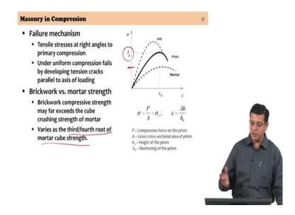
But if you were to examine the mortar, the mortar, the strength of the mortar in the masonry will be higher because of the triaxial confinement, the triaxial compressive stress in the state of confinement and will have a value, the compressive strength of the masonry will be significantly higher than the strength of the mortar itself. And this is because of the triaxial effect that is there the triaxial confinement that is there of the mortar.
