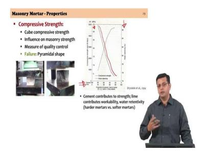
Compressive strength of mortar and again as a quality control test small cubes of mortar are cast in the site and tested, just as you would do quality control for concreting by casting those cubes or cylinders; cylinders in some other countries. So, the cube compressive strength is the parameter that we use both to classify the masonry mortar, earlier said MM 7.5 and MM 5, it is the cube compressive strength. And it is a small cube that is cast, it is a 50 mm x 50 mm side dimension.
