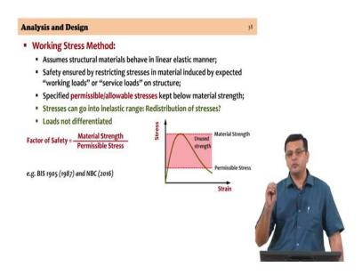
So, as all of you would be aware, working stress method has been the method of design for several decades and for several systems. Of course, today in our country, reinforced concrete design and steel design have migrated to limit state methods, but masonry continues to be operated under the working stress method.
