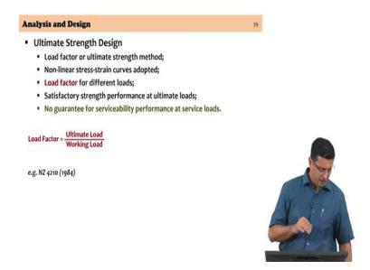
The ultimate strength design, which is a development after the working stress approach, is also referred to as the load factor method. In this load factor method, there is an implicit understanding that the stress strain curve of the material, in reality, is non-linear and in design we adopt a non-linear stress strain curve. So, there is a recognition of the fact that is in the behavior goes beyond the linear elastic range itself.
