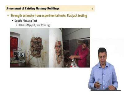
So, there are a couple of standards well established standards for how single and double flat jack tests can be estimated; can be conducted. One of them is the RILEM standards we were talking about RILEM in the previous lecture. It is a network of European laboratories and a number of test techniques are formalized through RILEM.
