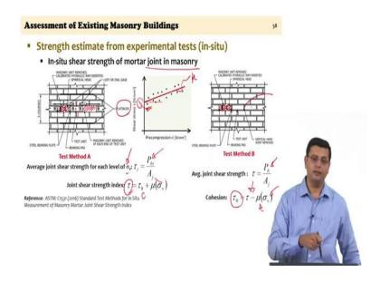
We talked about the difference between the masonry shear strength versus the shear strength of a mortar joint in masonry. Even that is a test that can actually be executed. Insitu it is less scarier than the previous test in terms of its requirements. But, you have standard test method here; I am referring to ASTM 1531. ASTM 1531 actually gives you the possibility of conducting this test in three different ways.
