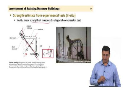
Continuing with in-situ tests, this first test is actually looking at compression behavior right. We looked at wallettes, we looked at cores which are looking at compression behavior. We looked at the flat jack tests which is again looking at a compression behavior right and deformability under compression.
