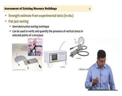
Continuing with the in-situ experiment tests, we will focus on a test called the flat jack testing today. So, the flat jack testing; there are two types of flat jack testing. You will appreciate the differences between the two types of testing depending on what you are actually looking for from the structure. The flat jack testing is classified as a semi-destructive test technique ok.
