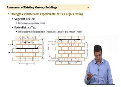
So, the single flat jack testing is meant to estimate what the in-situ axial compressive stresses. So, if I want to make an estimate of the, what is the vertical stress in a wall? Of course, vertical stress levels compressive stress levels are going to be different in different locations. So, you would make a specific choice on where you want to do this test and carry out this test.
