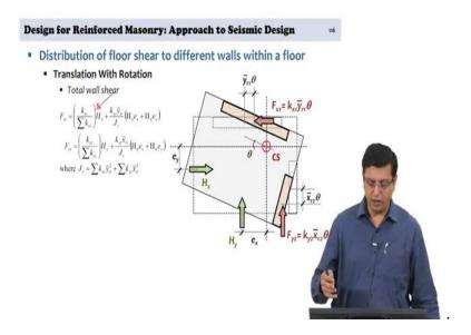
Therefore the total shear that the wall will experience is going to be. So, the shear force  $F_{xi}$  in wall 1 or wall 2 would actually be the translational component which comes merely by multiplying the shear force in that direction, in the direction that you are considering multiplied by the distribution factor that we saw earlier.
