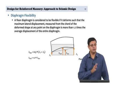
Having said that, I think it is important to examine for a moment, the role of diaphragm flexibility. Now, all this while we have been talking about a rigid diaphragm consideration. So, if you have a masonry structure, which has a reinforced concrete floor slab and roof slab; we are talking of a system that can offer adequate in-plane stiffness of the diaphragm. Mind you it is in-plane stiffness, it is not the out of plane stiffness which is the bending stiffness of the slab.
