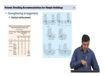
And finally, the vertical reinforcement; as far as a vertical reinforcement is concerned, this particular code caters to any type of masonry construction that you are working with solid units, hollow concrete blocks, the cement blocks, or even the hollow clay blocks.
