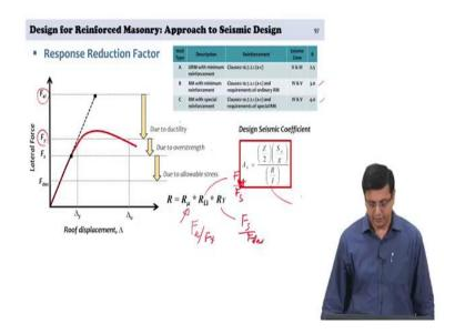
We will focus on the basis for design and then start defining the shear forces for the structure, the shear forces that are then distributed to the walls and from the walls to the piers. So, this process is what we are going to be examining here on, both for single storey and for multi-storey structures; however, this design is within the framework of earthquake resistant design.
