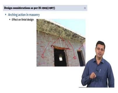
I have this very interesting photograph that tells you what is arching action and what is the load that the lintel will carry. And this is from one of the site visits this is the Indira Awas Yojana construction 6 meters by 4 meters construction using brick masonry and reinforced concrete floors you see that there is no lintel. Since there is no lintel you will have damage and damage in masonry, but it is very clear how the lintel should be designed only for that triangular load right.
