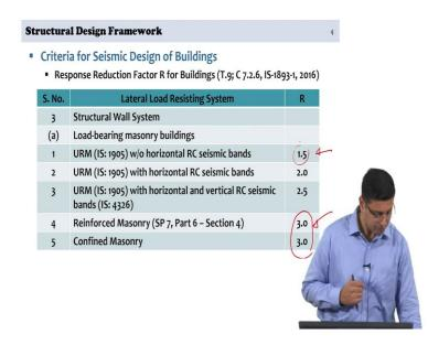
So, 3 a within this table that looks at response reduction factors, looks at load bearing masonry buildings ok. Then, it starts looking at reinforced concrete shear wall systems, but I am now interested in looking at the load bearing masonry constructions and as you can see there are 5 different categories provided under this ok. Let us read each of them. Unreinforced masonry classified as unreinforced masonry where the design is prescribed as per IS 1905 ok.
