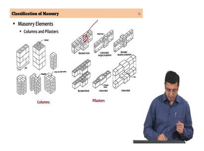
You also have columns and pilasters; the difference between columns and pilasters is the column is a single freestanding element of course, connected to the rest of the structural system. A pilaster is where you have a thickening of the wall like a small buttress and is
