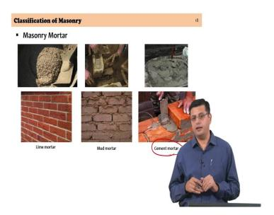
Mortar of course, this is again big spectrum, we have people who works specifically only on mortars in understanding their strength and durability characteristics. Mud mortar was predominant in the construction in the historic constructions, this is of composition that can vary from place to place and constituents that can vary from place to place. So, this is very non-uniform across the world and depends on traditional knowledge that region had in terms of the additives in the mortar itself.
