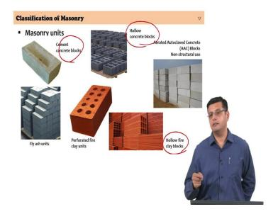
Continuing with masonry units, but modern masonry units, you have cement concrete blocks being extensively used today, you can, you can control, design strengths that you require, that uniformity in strengths you do not get with fired-clay bricks, you should be able to achieve it, but there is a physical challenge in achieving uniformity. The cement concrete blocks can give you that if the design I,s well if the mix is well-designed and quality control in the execution phase is there.
