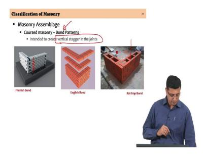
If you come to modern constructions the whole concept of coursed masonry and having a pattern is something that you would have definitely learnt in your earlier classes in materials. But the most important aspect is, to be able to create a vertical stagger in the masonry joints and this vertical stagger is essential for interlocking right.
