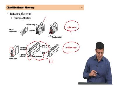
Beams and lintels in masonry can be constructed, but since beams and lintels are going to be dominated by flexure you have tension in them so you cannot construct them if they are flat, you cannot construct them using unreinforced masonry you have to reinforce them.
