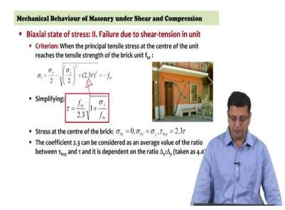
We will start we will look at the other two criteria one when the axial stress levels are intermediate. And you would expect that in a two storied, three storied masonry load bearing masonry construction in the ground storey and finally, a case where the precompression level is significantly high. So, the second criterion that we were examining was the shear tension failure in the unit itself.
