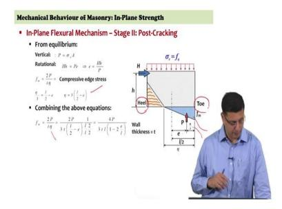
Stage II is post-cracking, post-cracking you have reduced cross section and now equilibrium is on the partial section of the cross section. So, the portion that has undergone uplift because of the direction of the lateral force, you refer to that as the heel of the wall, and the other end which is now experiencing higher pre-compression is the toe of the wall. So, you have toe going towards increased compression levels and can fail in crushing.
