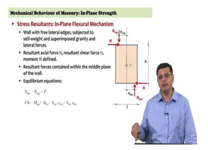
So, to start examining in-plane strength, we are now examining the in-plane strength of a masonry wall and again in a way similar to the different zones that we examined in the failure plane which was the end result of application of the Mann-Muller criterion, you had low pre-compression, moderate or intermediate levels of pre-compression and high pre-compression.
