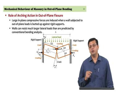
So, arching action is something that you can consider, under a given set of conditions, but if those conditions do not exist, it will be erroneous to assume that arching action is going to occur, because arching action can significantly increase the load carrying capacity of a masonry wall in out of plane bending.
