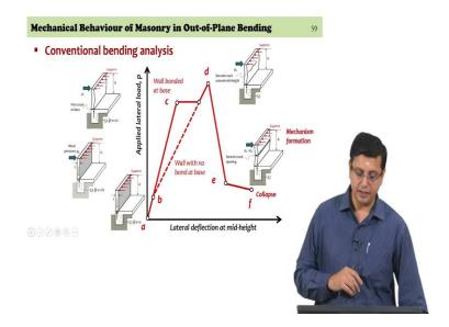
One; conventional bending analysis, where we are examining the section behaviour till ultimate as linear elastic and get the force displacement relationship based on introducing non-linearity in the way we want in terms of cracking occurring at the base and then cracking occurring at the mid height, but the section properties continued to remain linear elastic in compression that was one approach.
