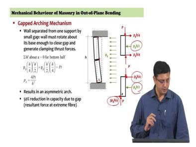
So, let us examine what would happen here, let us say there is a small gap at the top right, formed to do whatever reason, construction defect or shrinkage in the material and so on.
