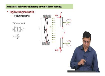
We will come back to that and see how some codes do give you the possibility of accounting for the arching mechanism, most others just depend on the conventional bending analysis itself ok. So, if we were to assume this initial case, where the non-moving supports are present, but there is no gap that exists between the wall and the support.
