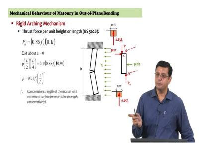
So, as I said it will be instructive to see how do codes account for this sort of a phenomenon that you can beneficially utilize in estimating the load carrying capacity of the wall in your design. So, the British code actually has a set of expressions that simplifies and helps in accounting for the arching action. It is BS 5628 that has this expression.
