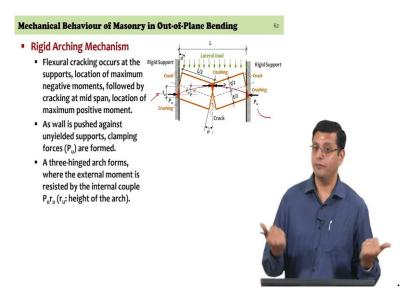
These clamping forces are what we are going to be trying to arrive at an expression for and these clamping forces as I said are actually, sitting at the centroids of the triangular area that is being considered at the ends of the wall that is a triangular area which is the one that is getting crushed and the contact area is now,  $\Delta_0$  there.
