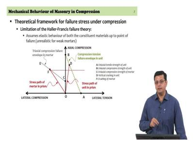
So, therefore, further developments in this direction have actually examined the possibility of looking at an inelastic behaviour of the mortar. This becomes an unrealistic, the elastic linear elastic assumption becomes an unrealistic assumption both for situations of the brick unit failing first or crushing happening in the mortar early on.
