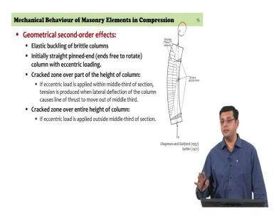
The assumption, the basic assumption that we make in this process here, we are looking at when you have eccentricity there is bending in the wall and that can basically lead to a situation of buckling. So, we looking at a brittle material masonry wall or masonry column and examining the phenomenon under elastic buckling itself.
