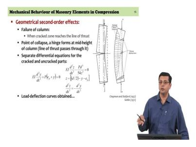
So, we will keep that in mind and use that as the fundamental difference between different resisting sections of the wall itself. The wall is expected to fail when the cracked zone reaches the line of thrust and that is at the moment of collapse itself you get a hinge that is forming at the mid height of the column the mid height of the column itself is the location where you have the maximum displacement and expect maximum cross section to have cracked.
