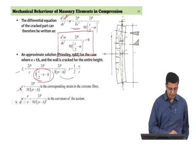
The curvature therefore, in the cracked zone is now written in terms of the curvature itself. So, we defined the total displacement eccentricity plus delta as  $\omega$ . So, the second derivative of the displacement as the curvature with now the expression for curvature derived as we saw in the previous slide is going to help us write down the differential equation for the cracked zone of the wall right.
