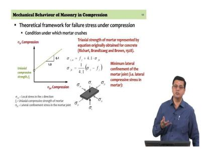
Now let us examine mortar and what happening to mortar, and we understand that when we are doing uniaxial compressive test on the mortar it is under uniaxial compression, but in the prism under compression the mortar goes into state of triaxial compression. So, you need to alter the uniaxial compressive strength of the mortar to be able to explain what strength you would get in mortar in a confined manner right.
