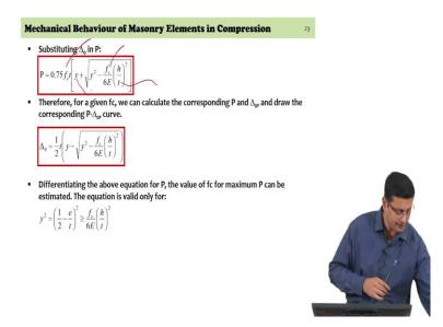
So, if we were to assume the curvature along the height being constant then the double integration becomes simpler you get from the expression for the curvature at any section plug in the values solve it and plug in the values and you get an expression in P. So, you get with this simplification you are able to pull out an expression in P you need a load displacement you need a load displacement finally, to be able to draw the effect of eccentricity of the load itself.
