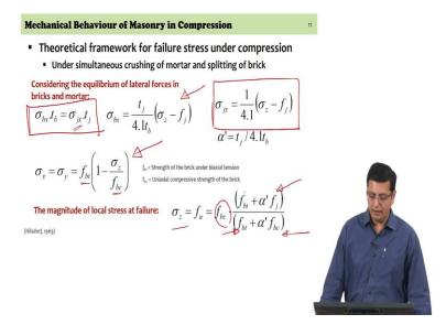
So, with the failure planes for the constituents defined if we assume that now these two phenomena are meant to occur together; that is the crushing of the mortar is happening as soon as or immediately after the splitting of the bricks in the bilateral tension. Then we use our original equilibrium equations and rewrite the expressions that we saw in the previous slide to be able to pull out an expression for  $\sigma_z$  now from the material constituent strengths themselves.
