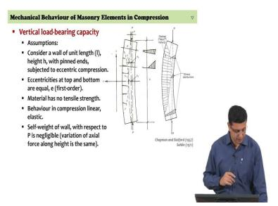
So, let us examine this we want to calculate the vertical load bearing capacity of the wall and these are the assumptions that we begin with. We are considering a wall of length l; height h, it has pinned ends and it subjected to eccentric compression. We have the same eccentricity at the top and the bottom; eccentricity represented with the notation e here top and bottom eccentricities are equal.
