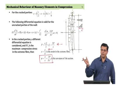
If eccentricity is greater than; if eccentricity is greater than t/6 then we have to then estimate what is going to be c which is less than t. Now for the cracked portion we look at a trianglur distribution the width of the compressed zone is c, the total length is t and we want to estimate what is this width of the cracked zone in case the eccentricity is greater than t/6.
