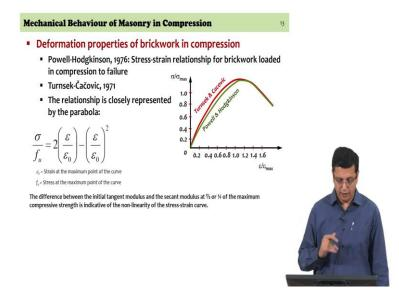
So, continuing it is useful to look at in terms of stress- strain curve what sort of what sort of a analytical formulation fits the stress-strain curve of masonry itself. Again ,we are examining compression and in a way it is not very different from concrete in its behaviour in compression and studies were carried out few decades ago and they still valid because they do a rather good job in capturing the stress strain behaviour of masonry in compression.
