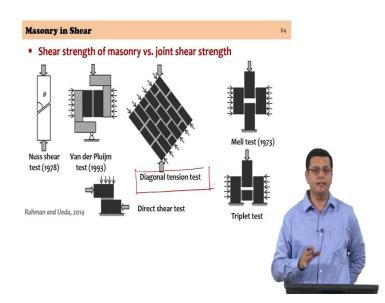
Fundamental aspect that you need to keep in mind is when you are examining the shear strength of masonry you will have to distinguish it from the joint shear strength. The joint shear strength is dealing with the bond between the units and the mortar. So, the joint shear strength establishes the strength present in shear between the unit and the mortar. The shear strength of masonry is affected by the joint shear strength but is not the joint shear strength, ok.
