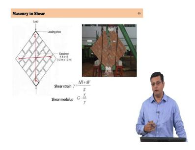
So, if you were to examine the failure pattern you can see the line of tensile cracking parallel to the line of application of the compression and as you can see in this particular figure in this particular picture, you have a combination of line and unit failure. So, the bed joints typically are stronger than the head joints. Yes, the bed joint is the horizontal joint, the head joint is the perpend or the vertical joint between the brick units.
