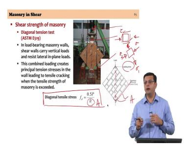
So, let us first examine the diagonal tension test and we are actually characterizing the shear strength of masonry with the diagonal tension test. There is an ASTM standard, we do not have an Indian standard that regulates the testing under the diagonal tension condition, diagonal tension test condition. The ASTM standard E519 gives the protocol for testing. It is also referred in the literature as a diagonal compression test and in a moment you will agree with me why the nomenclature.
