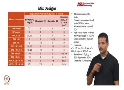
So what we did is, with the available materials we designed a large number of systems of paste mixes, actually 33 in this study, very low water binder ratio 0.24, we actually went down even further, 1.25 percent of high range water reducing admixture, a polycarboxylate base water reducing admixture, 1.25 percentage of solids by mass of binder which actually translates to about 5 percent of super plasticizer by mass of cement, 5 percent I will show you how to add that also.
