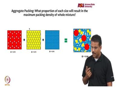
Now aggregate packing, so how do you do aggregate packing? If I have one size of aggregate, the best I can do with small size aggregates is to get a packing fraction of 0.91. But if I start
