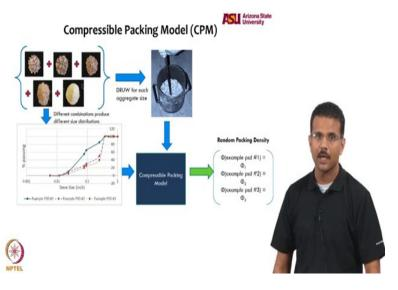
So here is a compressible packing model, get all the different sizes of aggregates that you want, get the dry rodded unit weight for each of those class of aggregates, put all of them in the compressible packing model along with particle size distribution, come up with random packing densities, if you do that you will get random packing densities.
