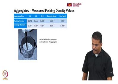
And then you have to find out the measured packing density of each of the aggregate classes. This is the only lab experiment that you have to do for that, for each of those sizes you find out what is the actual maximum packing density by doing a dry rodded unit weight test in the lab and that will give you a maximum packing density.
