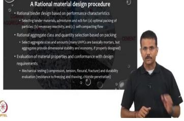
So how do we design this material? How do we start designing it from first principles? So you have to select what binder materials you actually want and that is the most important part. Cement is a given you need it, what other than cement? What are the common ideas that we have to select a material other than cement? One is sustainability, you have to make sure that you are using less cement as possible so you can use lot of other base materials.
