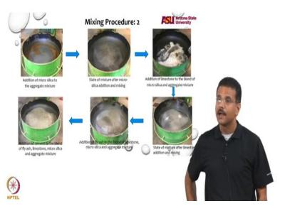
Silica fume is added first to break down the silica fume agglomerates. So you put the silica fume in and make silica fume dispersed by mixing and then add the limestone because limestone are the next larger size. Then you mix this well so that you get a good mix and then add fly ash.
