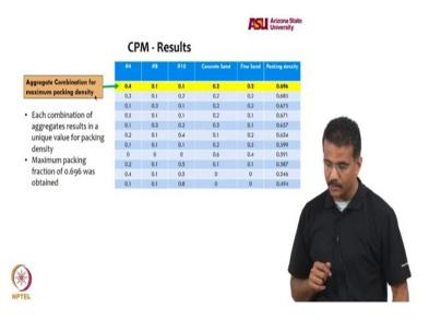
Based on those combinations pick up the one with the maximum packing density, in this case it is 0.696 where I have 40 percent of number 4, 10 percent of number 8, 10 percent of number 10, 20 percent of concrete sand which is 0.6 mm and 20 percent of fine sand which is 0.2 mm. Now
