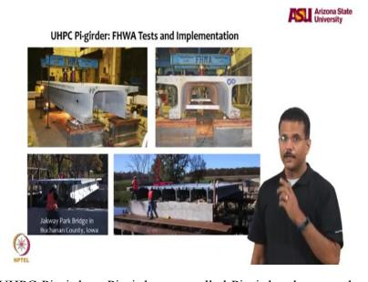
These are again UHPC Pi-girders, Pi-girders are called Pi-girders because they have a shape of the Greek alphabet Pi and these are very common bridge girder elements. So Pi-girders are very common. You can see Pi-girders being implemented in Jakway Park Bridge in Iowa.
