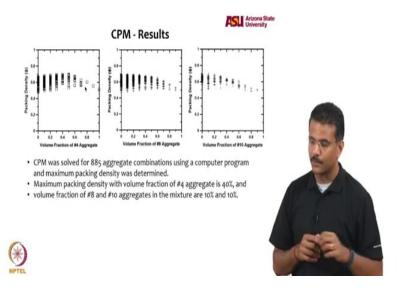
This is some plots for 885 different aggregate combinations, MATLAB code will do it in 2 seconds, and then you plot the random packing density as a function of volume fraction of different aggregates and you can find out where is a maxima in the packing density for different combinations.
