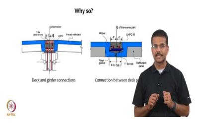
So we will attack this problem in two different stages like I said two different ways of doing, you can deck and girder connection or you can have connection between deck panels you can see the reinforcement in both cases being different.
