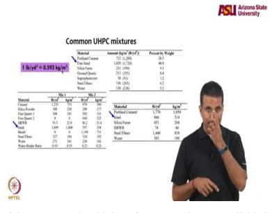
So here are some of the common ultra-high performance mixtures available in the market. There are mostly commercial mixtures, I have put the conversion between pounds per cubic yard and kilo grams per cubic meter for you to quickly make the conversion and the first thing that you notice is very high amount of cement.
