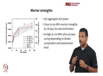
We did mortar strength and you can see that we can get upto 150MPa strength at 28 days. This is 35 percent aggregate and 65 percent paste, that is not a typo you normally see it the other way in mortars and concrete, you need that amount of paste to satisfy the workability and the strength criteria and we get 170 MPa after 90 days with all these mixes which have 30 percent cement replacement. So that is fairly good.
