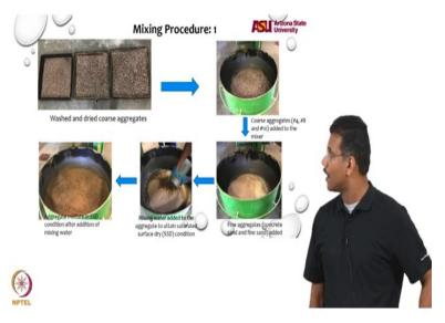
So aggregates are washed and dried, aggregates are added to the mixer, fine aggregates are added, mixing water is added to the aggregate to attain a saturated surface dry condition and then mix it together and blend all the aggregates together, and add silica fume first.
