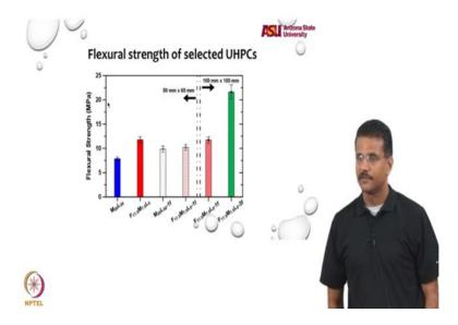
If you look at the flexural strength, 20 to 25 Megapascal flexural strength for these materials, if you have it fiber reinforced extremely high flexural strength.
