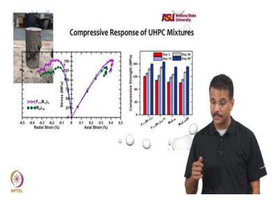
So here is the complete axial stress axial strain and axial stress radial strain curves for non-fiber reinforced UHPCs. You see the maximum strength is 150 Megapascal, the maximum axial strain is of about 0.3, 0.35%, which is basically the maximum allowable strain of concrete in the sign. So first understanding is that the ultrahigh performance concrete does not change the maximum axial compressive strain capacity of concrete in unreinforced state.
