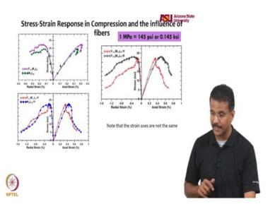
Now, when you look at the influence of fibres, this is a little tricky figure because the stress axis is in kips per square inch which is 1000 psi. So the left top figure is the same one that I showed earlier, which is basically the axial strain and radial strains as a function of axial stress for unreinforced mixes and the one on the left bottom is for a mix with 1% fiber.
