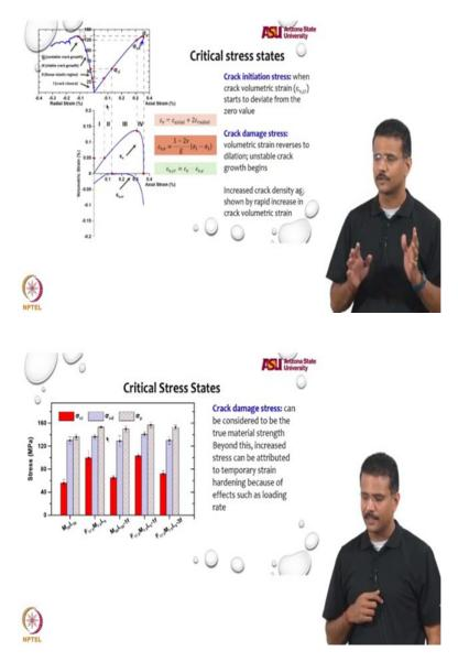
Now, slightly more different structural aspects to think of when you design this mix. What I have shown in the picture on the left top are the stress strain curves, but marking significant points on stress strain curve based on the strain relationships, so what if the bottom curve are the axial strain versus volumetric strain.
