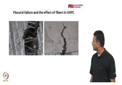
Effect of fibres, again you will see fibres bridging the cracks, a lot of fibres in flexural failure.
