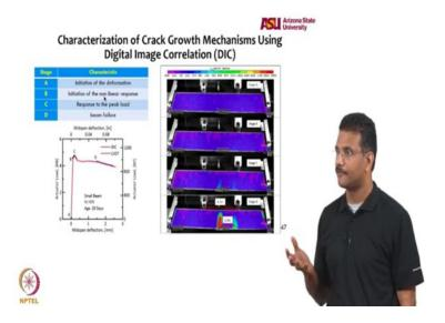
So just to give you a few important points in the load deformation plot, if you see the top picture, stage A corresponds to just the starting loading pattern, you have almost no strains setup in the material, whatever you see those pink strains at the edges are of the compression of the loading support. It is not really the effect of loads but you just start to see some patterns of strains emerge.
