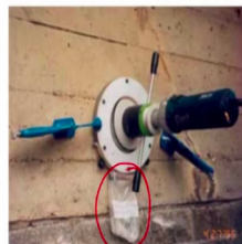
Powder samples being collected directly from the field structure
