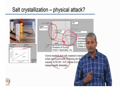
Now one aspect that you see in the field often is salt crystallization, which exerts a bits or deteriorates a concrete much further, okay and again this example of the soil air interface was primarily because of the salt crystallization problem, certain forms of sulphate like sodium sulphate can transform into hydrated forms like (mirabilite) thenardite to mirabilite transformation and this happens within these restricted pores spaces of your system, okay.
