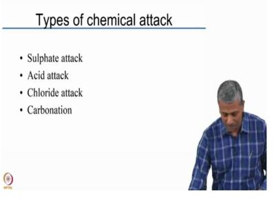
Now there are generally several other type of chemical attacks apart from sulphate attack also. For example you may have acids attacking concrete, you may have chlorides directly attacking concrete as in the case of sea water, and sometimes even in ground water there might be the sources of chlorides and the other chemical attack is carbonation that is attack of concrete by atmospheric carbon dioxide.
