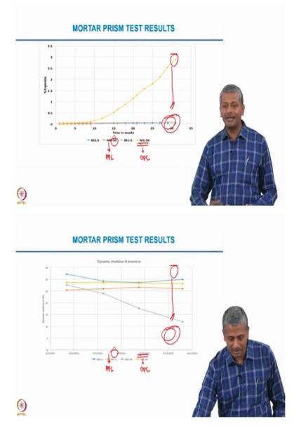
You can see the expansion results here in terms of this M1 basically relates to Ordinary Portland Cement and M2 relates to portland pozzolana cement so that has got fly ash in it 30 percent fly ash in it, okay. So M1 at 50 gram per litre is showing a significantly high expansion close to 3 percent after about 32 weeks of exposure, okay these are weeks of exposure.
