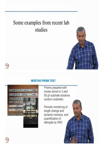
Some examples from recent laboratory studies just to put this in perspective so here these are mortar bars which are stored in different concentration of sulphate solutions 3 gram per litre and 50 gram per litre of sodium sulphate solution and periodic monitoring of the length change was done, also dynamic modulus by resonant frequency was determined for this mortar bars.
