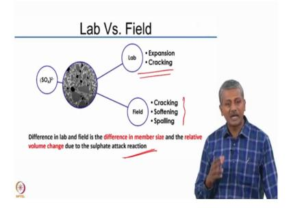
Now again let us look at lab and field for a minute again, I talked about the fact that in the lab we have smaller scale specimens they are usually continuously immersed or sometimes we may introduce variations like wetting and drying, okay but there is no way that you are ever going to able to simulate real life environment in the laboratory, okay. So let us look at something little bit in more detail.
