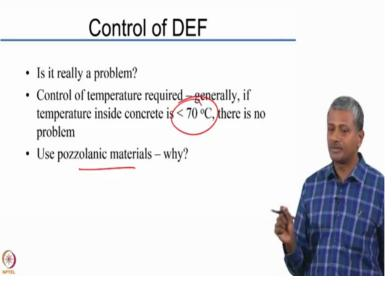
Now control of DEF of course we have to understand whether it is really a problem depending upon the situation it can be a problem, if you have very high temperatures during precasting so generally because of that most concrete it says the specification for concrete construction typically put a limit on the maximum temperature permissible inside the concrete.
