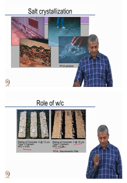
So interestingly this is still something which we observe this is examples of salt crystallization and again data from portland cement association which clearly show that compared to a high water cement ratio system a low water cement ratio system even after 16 years had a very high visual rating after being exposed to very aggressive sulphate solutions, okay. So again the control of water cement ratio happens to be the most critical aspect as far as sulphate is concerned, okay.
