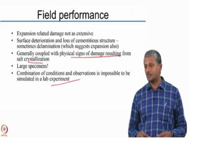
So in field you see that expansion related damage is not extensive because small skin expanding on the surface will not result in a major cracking of the system. Surface
