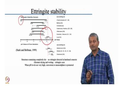
Again as far as stability of ettringite is concerned the stability domain is restricted to certain pH. So for example in highly acidic solutions like sulphuric acid for example you will probably will not have any ettringite unless you go deep into the structure of the concrete, in the surface zones where the acid has already penetrated you will probably not be able to crystallize ettringite because it is not stable in that domain.
