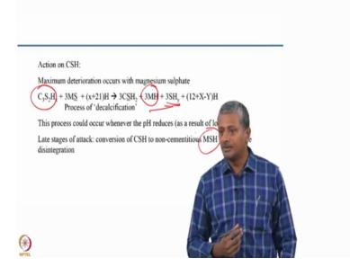
So what happens ultimately is your C-S-H can decalcify and lead to the formation of something like a silica hydrate. Now silica hydrate does not have the same binding characteristic as your C-S-H, okay and soon this magnesium which is present as a magnesium hydroxide can combine with the silica hydrate to form what is called magnesium silicate hydrate MSH magnesium silicate hydrate then absolutely that is absolutely got no binding
