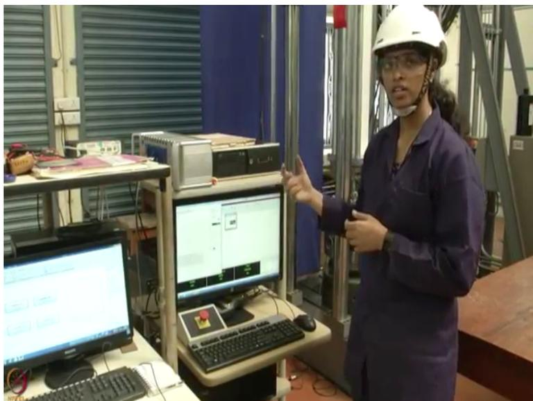
So we have connected the LVDT to, two LVDTs and the load cell of the testing machine, actuator of the testing machine to the external data logging system where the data will be recorded during the testing.
