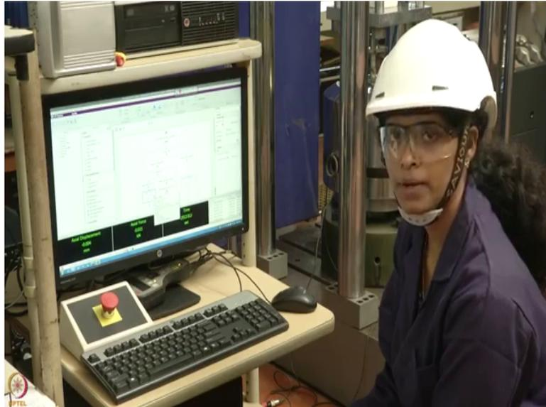
So once those setups are done, we have a customised test program for running the pull out test for prestressing strands, so these are the procedure for the test program and before starting the test ensure that LVDTs position are at zero if not offset the reading to make it zero, so this is the test program customised for pull out test for prestressing strands, so where this program is based on closed-loop testing where load will be applied at the rate of 2.5 MM per minute.
