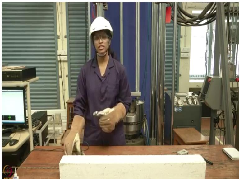
Then we will mounting pull out specimen here, so we are now going to place this specimen on the frame, you have this 350 MM expose the strand at this end and 150 MM expose the strand at the other end, so this end will be placed at the bottom and it will be gripped and that
