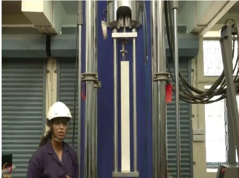
Now we have fixed the pull out test specimen on the frame and place the one LVDT at the load at end, it is called live end where load will be applied and another LVDT at the top, free end and the specimens are whitewashed using a Plaster of Paris to absorb any crack developing during the pull out test and it is move on the testing.
