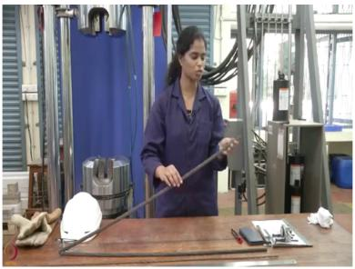
Typically three types of strands are being used in pretension or prestressed concrete systems, those are 3wires trends which has 6 MM diameter and next one 7 wires strands with 12.7 MM diameter which is typically used in pretension concrete systems and the next one of 15.2 MM diameter stands again this was also 7wire stands which is typically which is typically used in post-tension concrete structures.
