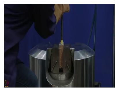
We had this universal testing machine from MTS, the machine capacity is 1000 kN which is fully servohydraulic control and this is the hydraulic control system which will be used to apply the lateral pressure for gripping the strands and this controls we have to moves this upper portions to place the strands, now we have place the strand under the machine for the testing, once the strand is fixed preloaded is applied to give the strands straight.
