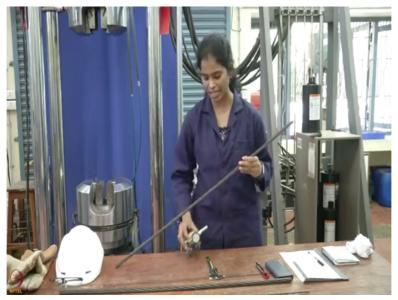
So basically strand is at of 7wires, 6 outer helical wires and 1 centre king wire, so to get the correct area of the strand, you need to measure the individual outer diameter of the strand and then king wire and some of that to get the actual area of the strand, so you have to measure the nominal diameter of the strand using vernier caliper, then we can measure the pitch length
