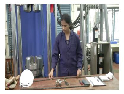
So once the gauge length is fixed we can prepare the gripping portion of the strand, so we need to, so for any tension test gripping is very important because we need to avoid stress concentration near the wedges, so basically when we apply lateral pressure while gripping that will induce test concentration and that may affect the result.
