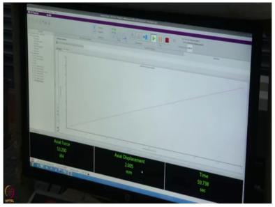
So while test is running here you can see the load displacement behaviour of the strand and now you can see the load is linearly increasing and the force and the displacement are showed at the bottom of the screen, meanwhile reading will be taken, dial gauge reading will be taken
