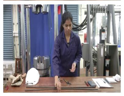
So now we can start doing the testing for 7wire stands, before starting the testing we need to do the specimen preparation and certain measurements for the calculation purpose later, so we need to have vernier apparatus to measure the nominal diameter of this strand and we have dial gauge to measure the elongation of the strand during the testing and we have the skill to measure the length of the strand before replace the strand in the testing machine.
