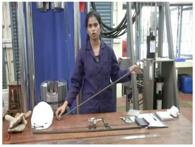
So you can see the groups made on the plate on which strands will be placed and during testing we may face some slipping, so to avoid that ASTM specifications as given to, suggested to use aluminium oxide oil slurry made using glycerine and we have placed the clamp at both ends make sure that the, this strand is not slipping or rotating during the testing.
