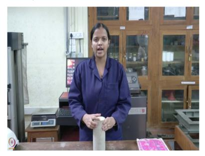
The specimen should be grinder or capped before testing, in order to make sure the surface is smooth otherwise there will be irregularities in the specimen because of casting and stress concentration might occur and you will not have uniform loading on the specimen.
