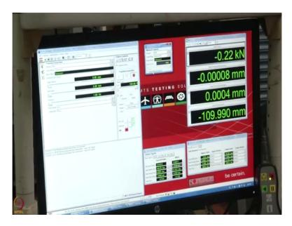
So first the controller has to be switched on, after that will open the software called Station Manager which will control the testing, so this is the software used for the testing, first let to switch on this exclusive control, so that we can use these two icons, first we will switch on the hydraulic power unit which supplies the oil to operate this machine, then will be switching on the HSM.
