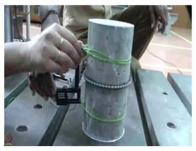
So the when end of the chain will be attached to the extensometer and will place the chain around the specimen, now we have to elongate the extensometer, so that we can connect the other end of the chain, check whether the chain is kept at the centre of the specimen, will place the extensometer on the markings, so by using a rubber band we are fixing the extensometer in-place.
