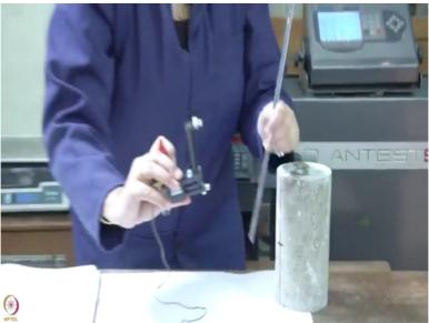
So before starting the test you have to measure the diameter, initial original diameter of the specimen and we are measuring the height of the specimen, now we have measure the height and diameter of the specimen, now I will mark the specimen to attach the extensometer, so we draw a straight line and will mark the centre of the specimen, in a case it is 195 MM, so I will be marking the centre of the specimen, then in order to attach the extensometer, the extensometer gauge length is 100 MM.
