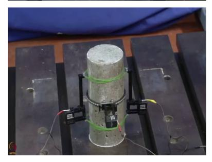
The blades of the extensometer should be placed on the markings, similarly we are placing the another extensometer, while placing the extensometer make sure the pin on the extensometer and before starting the test, you have to remove this pin, so that the extensometer deforms.
