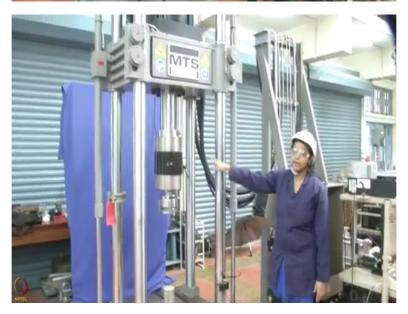
So this is the closed-loop testing machine in which we will be doing the compression test, this cross cade can be manually moved by means of this manual controlled lever arm, the capacity of the machine is 1000 kg newton, which is powered by hydraulic unit, the actuator can be moved with the help of the software in the system, so you, we also have a LVDT above the actuator, which measures the movement of the piston, now you will attach the extensometer on the specimen.
