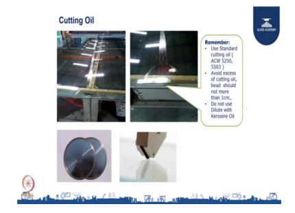
Cutting oil, so, cutting, how effectively can use it basically the amount of cutting oil if you use less the cutting oil uses only for cutting the glass alone, we should not spread like more than 10 centimeters. So, you can see that widespread, basically you are wasting your cutting oil.
