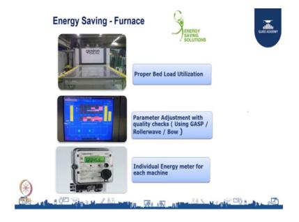
And energy saving in furnaces, proper bed load in utilization basically, when you plan a tempering in production, how you how can do in start the production you hope you are understand. First you have to start the, the higher thickness where the temperature is less temperature is required to temper the higher thickness of the glass. So, basically you have to put a first 12 mm, 10 mm, 8 mm, 6 mm, 4 mm.
