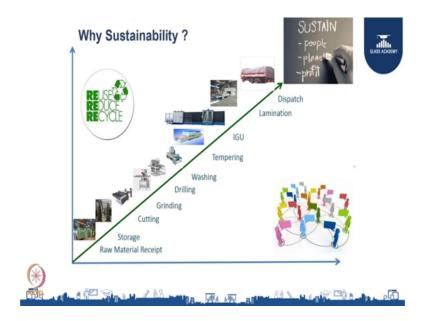
Why Sustainability? Will have to reuse reduce recycle of products. So, raw glass receipt, storage, cutting, grinding, drilling, washing, tempering, IGU, lamination and dispatch. So, these are the typical processing line. So, where all you can achieve this sustainability, that is all we are going to talk about now.
