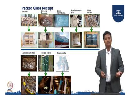
Next, you will move on to packed glass receipt so, basically packed glass would have a wood. So, naked glass would not have a wood so, that is the most important point which have to look at here. So, these woods like a nyle, endcap know this a endcaps and blue polythene reclaimable pads steel straps for you know winding the surfaces from manufacturer to processor, this would have, would have noticed the steel strap have been tied on over of the wooden pile.
