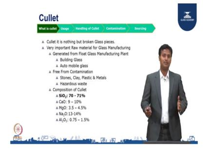
So, what is cullet? Cullet is nothing, but broken pieces it is very important raw, raw material for a glass manufacturing. So, all the processes should understand that what are the glass breakages you have so, that can be recycled. So, if you properly keep it on respective place, you split into the coated, non coated, basically a clear glass then there
