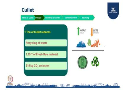
Usage 1 ton of cullet reduces recyclic of wastage, ok. We can recycle the complete wastages what we have as a broken pieces. 1.5 ton of fresh raw material if you have, it is just you know such a huge resource for raw glass processing. And this is reduction of you know I mean a 315 kg carbon dioxide emission it helps. Basically, it do not want to burn the fuels such as like this you can get it through this.
