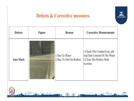
Now, let us understand one by one. Line mark, reason is very simple, quality of water or due to dirt on rollers. Corrective measure is check the conductivity, pH and salt content of the water; clean the rollers with acetone and you can avoid line mark.
