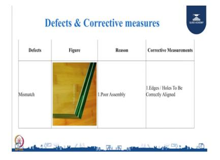
Mismatch, the reason is very simple, poor assembling. When two glasses are not properly assembled then mismatch will happen. Correction corrective actions are edges and hole to be correctly aligned, a simple method you can avoid mismatch.
