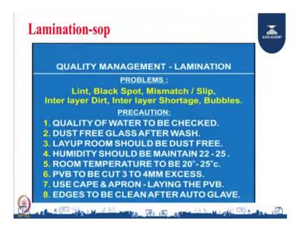
It is a general check list you must have to avoid lint, black spot, mismatch, slip, inter layer dirt, interlayer shortage bubbles. Quality of water to be checked; dust free glass after wash, lame room lake room should be always dust free, humidity should be maintained in 22 to 25 degree. Room temperature should be 20 to 25 Celsius; PVB to be
