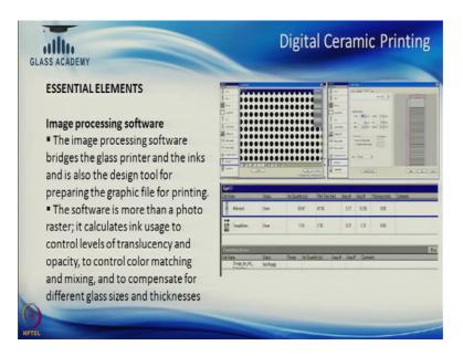
So, the image processing software will calculate that for you, as it is shown over here what is the dot coverage, what is the amount of ink that is going to be used. Since you are able to calculate the ink that you are going to use, you can calculate the cost per print. As I explained earlier, the inks are really expensive for the digital prints, but they cover a lot more area, why? Because the inks are really thin.
